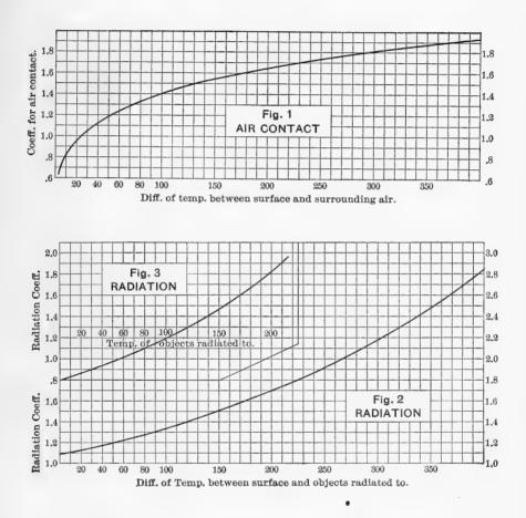
The loss of heat by air contact depends on the diameter of the pipe, on its position, whether vertical or horizontal, and on the difference of temperature between its outer surface and the surrounding air. We may express it by the following equation:
