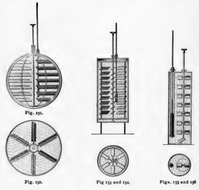
are very thin and of fir wood; they project into very small metallic appendices soldered to the vessels. When the cylinders are placed horizontally, the stem of the agitator turns in a cork which closes the tubular opening. There is a little play between the stem and cork, but the water does not escape on account of the expansion of the small quantity of air remaining in the vessel. This expansion is due to the contraction of the water by cooling.
