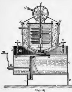
has within it a copper tube bearing paddles at different heights and having at its lowerenda horse hair brush. This tube is guided by two rings secured to it by the rods II and I'I' and it bears at its upper end a pinion driven by means of the gear and crank M'.
