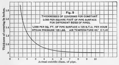
The useful lesson to be drawn from Figure 9 is that the loss of heat from small pipes will always be large in proportion to their surface, and it is also to be remembered that the proportion of surface to weight of steam passed is much greater for small pipes than for large.
