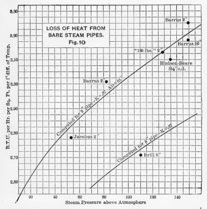
allows for the different loss of a different size of pipe, but Barrus test on the 10-inch pipe is equally strong evidence that it does not. Hudson-Beare's test also agrees with the theory.
