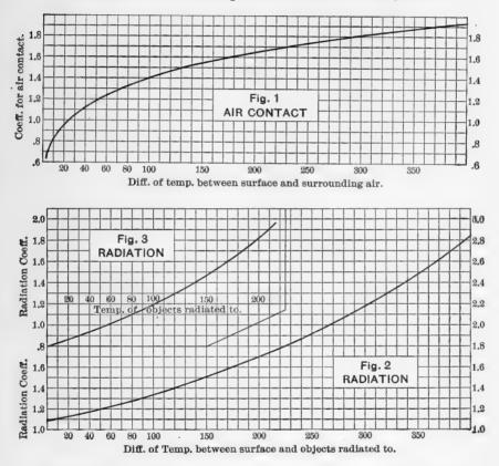
the nature of the surface of the body, and of the absolute temperature of the surrounding air; it depends solely on the excess of temperature of the surface of the body over the temperature of the surrounding air, and on the form and dimensions of the body."
