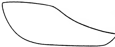
Fig. 257. Indicator Card with Exhaust Lap too large.
