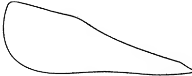
Fig. 255. Indicator Card with Steam Lap too large.
