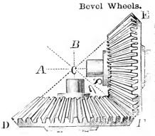
If the lines C A and B C represent the prolonged axes, which are to revolve with different or similar velocities, the position and sizes of the wheels for driving these axes are determined by the distance of the wheels from the point C. The di-
