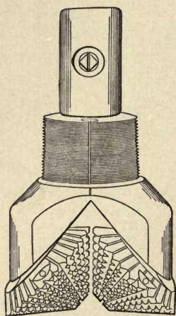
FIG. 77.—Sharp & Hughes hard rock rotary bit.
