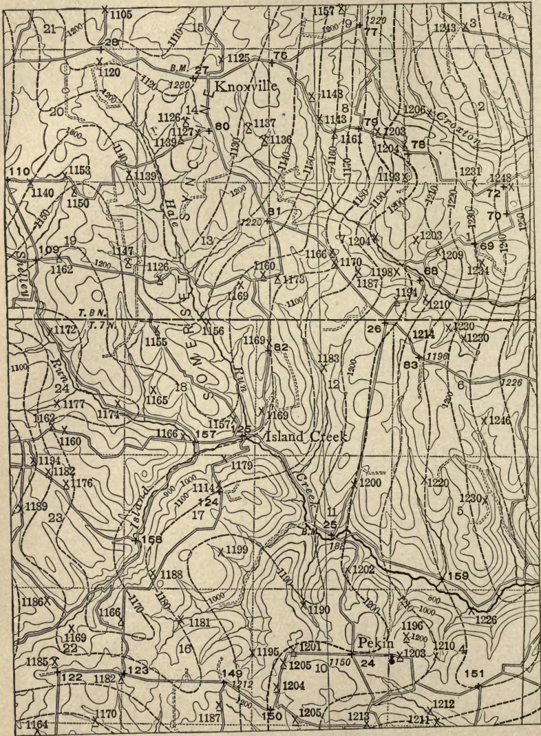
FIG. 48.—Contour Map of Key Horizon, which in this case is the Pittsburgh Coal.
