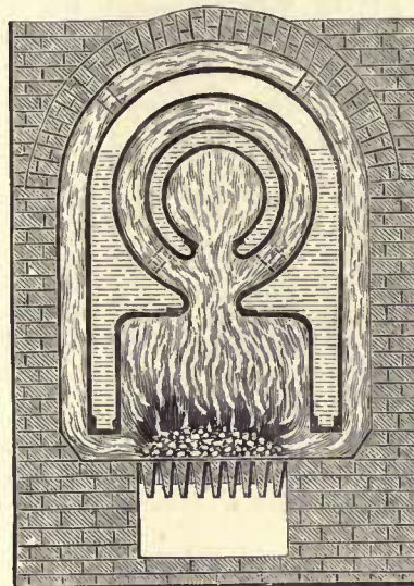
Ormson's Horizontal Cast Wagon Flue Boiler, shown in transverse sectional elevation. Patented in the year 1869.
