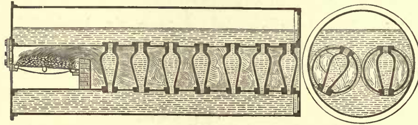
Arnold's Horizontal Cylindrical Boiler, containing two flue tubes fitted with pear-shaped water tubes. Patented in the year 1868.
