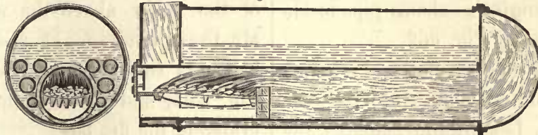
Napier's Locomotive Boiler, being a cylindrical shell with a cylindrical flue tube, semi-globular combustion chamber, and return flame tubes on each side of the flue. Patented in the year 1831.
