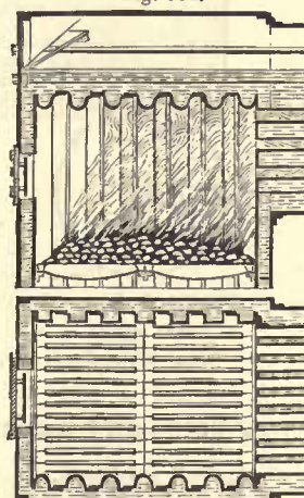
Dunn's Locomotive Fire Box, having a corrugated crown and sides. Patented in the year 1853.
