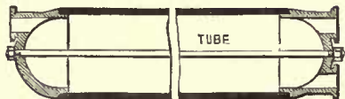
Dunn's Method of securing the ends of a tube with a bolt and nuts. Patented in the year 1853.
