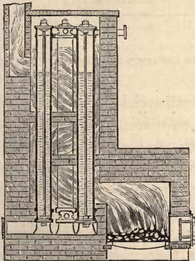
Jordan's Vertical Tube Boiler, set in brickwork. Patented in the year 1865.
