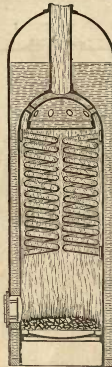
Selby's Vertical Cylindrical Boiler, fitted with water coils and a top water box. Patented in the year 1861.
