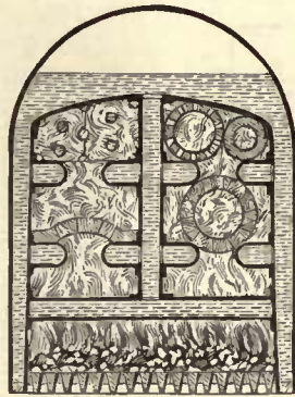
Transverse Section of Beattie's Locomotive Fire Box, fitted with central vertical and transverse horizontal water spaces, and also projecting water spaces supporting perforated brick retorts and slabs. Patented in the year 1855.
