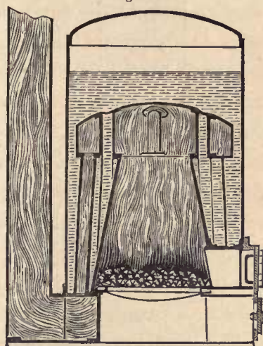
Cater's Vertical Cylindrical Boiler, fitted with flame and water tubes, and side chimney. Patented in the year 1861.
