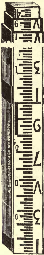
FIG. 127.—Staff with intermediate foot readings.
