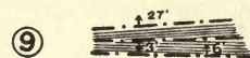
FIG. 147.—Usual methods of delineating underground workings, etc. (1) Arrows indicating air-currents; (2) air-crossing, overcast and undercast; (3) pillars and stalls; (4) stopping; (5) door; (6) sheet; (7) pit-shaft; (8) regulator; (9) faults and faulty ground.
