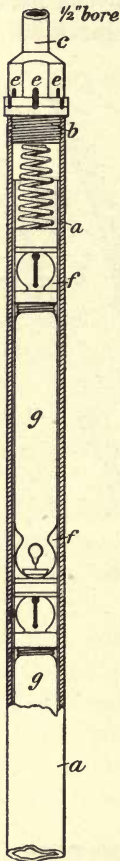
FIG. 172.—Macgeorge's instrument. Section, showing guide-tube in bore-hole, with the clinostats in position.
