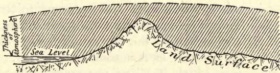
FIG. 137.—Theory of barometric levelling. The shading represents the atmosphere.
