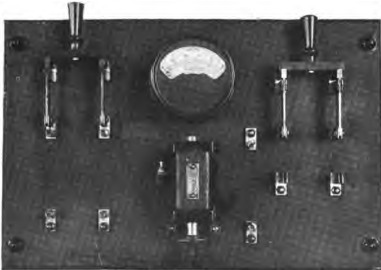
Fig. 205a—Charging Panel Used with Marconi Tuned Coil Sets.
