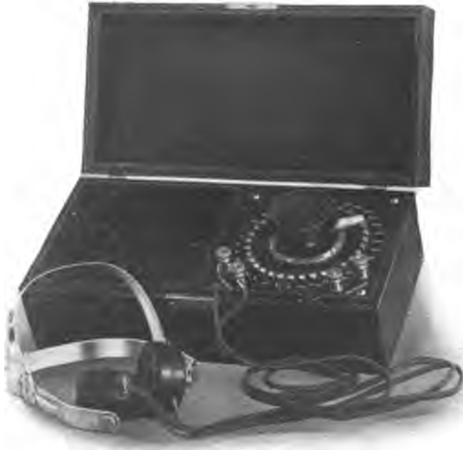
Fig. 238—Audibility Meter (American Marconi Company).
