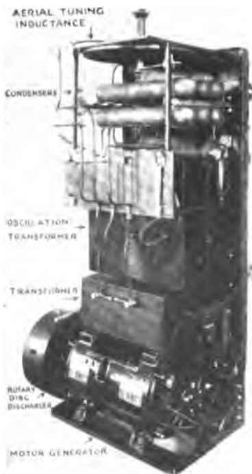
Fig. 265—Rear View of the Marconi \frac{1}{2} K. W. 120 Cycle Transmitter.
