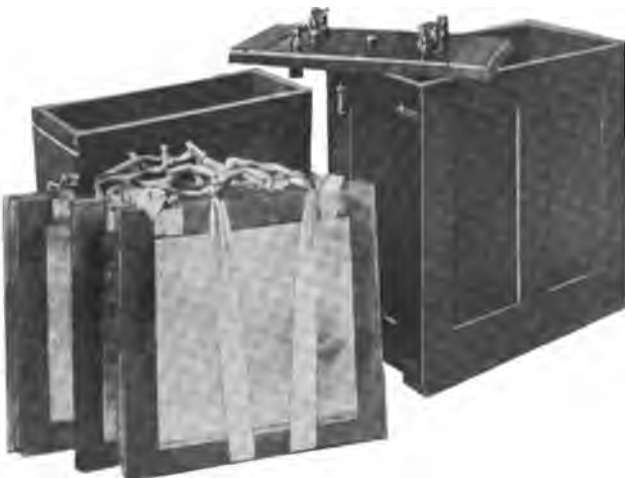
Fig. 129a—Marconi Glass Plate Condenser
