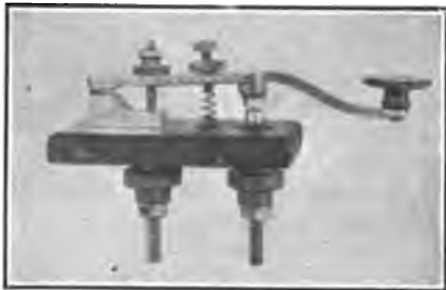
Fig. 137—A Hand Manipulated Telegraph Key.
