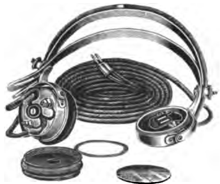
Fig. 194a—3 000-Ohm Head Telephone Receiver.
