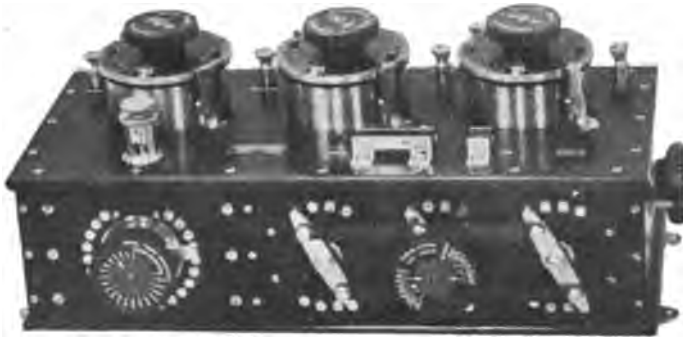
Fig. 167a—Marconi Multiple Tuner.
