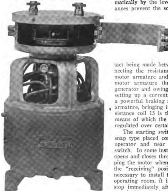
Fig. 75—English Marconi Company's one-half Kilowatt Vertical Type Converter with Synchronous Disc Discharger on Shaft.
