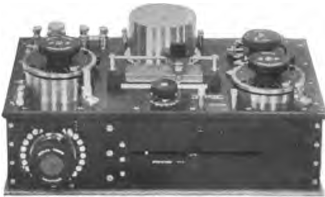
Fig. 177—Universal Crystal Receiver (English Marconi Company).
