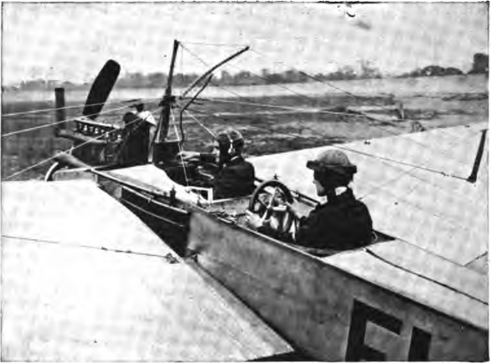
Fig. 325A—Scout Airplane Equipped With Wireless Apparatus.
