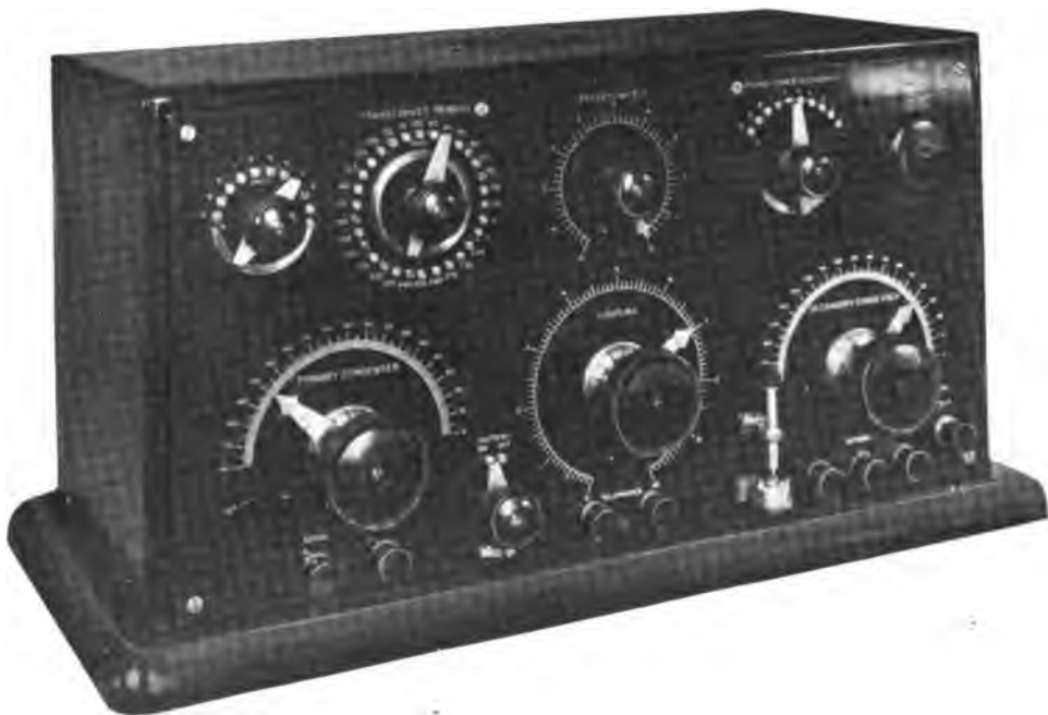
Fig. 170—Type 106 Receiving Tuner (American Marconi Company).
