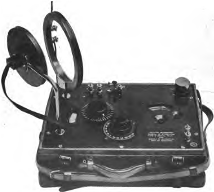
Fig. 221—Kolster Decrementer—the Type Used by the Government Radio Inspectors.
