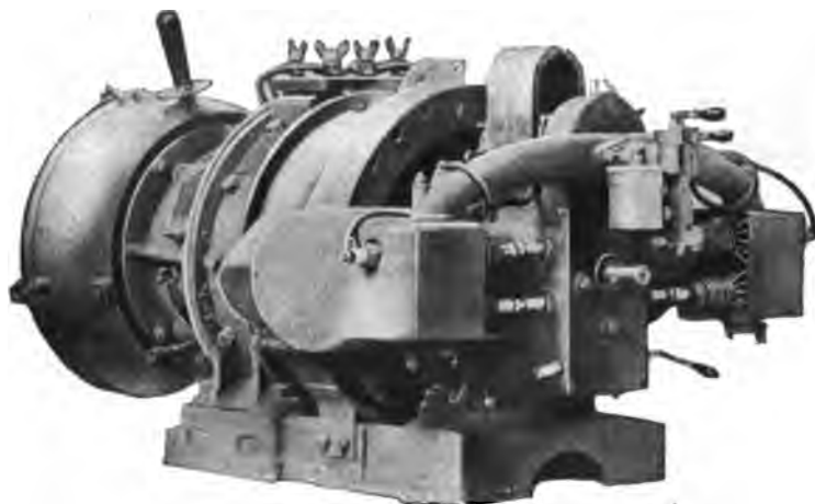
Fig. 10a—Combined Gasoline Engine, Generator and Disc Discharger for Portable Wireless Stations.
