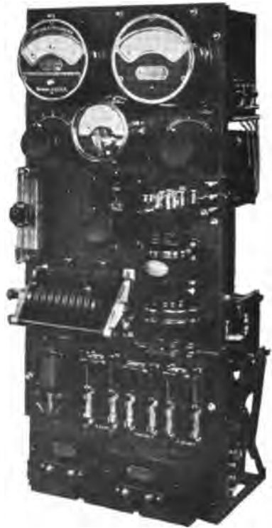
Fig. 250—Special Submarine Type Panel Transmitter (American Marconi Company).
