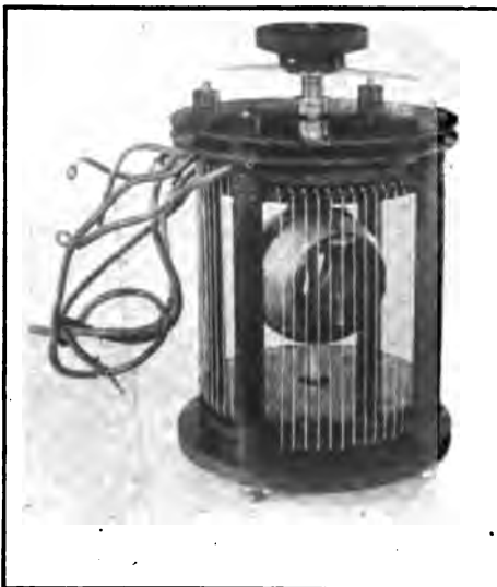
Fig. 272—Detail of the Radio Goniometer.
