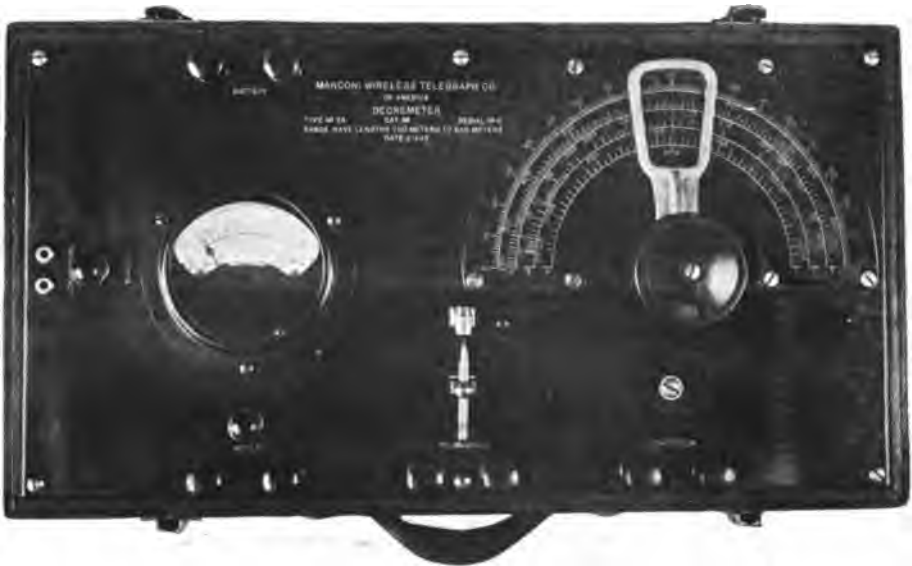
Fig. 220—The American Marconi Company's Decimeter.
