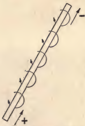
Fig. 12a—Showing Lines of Force Around a Conductor with the Current Flowing Away from Reader.
