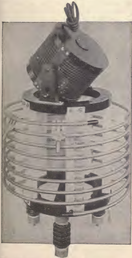
Fig. 119—Type A Oscillation Transformer of the American Marconi Company.
