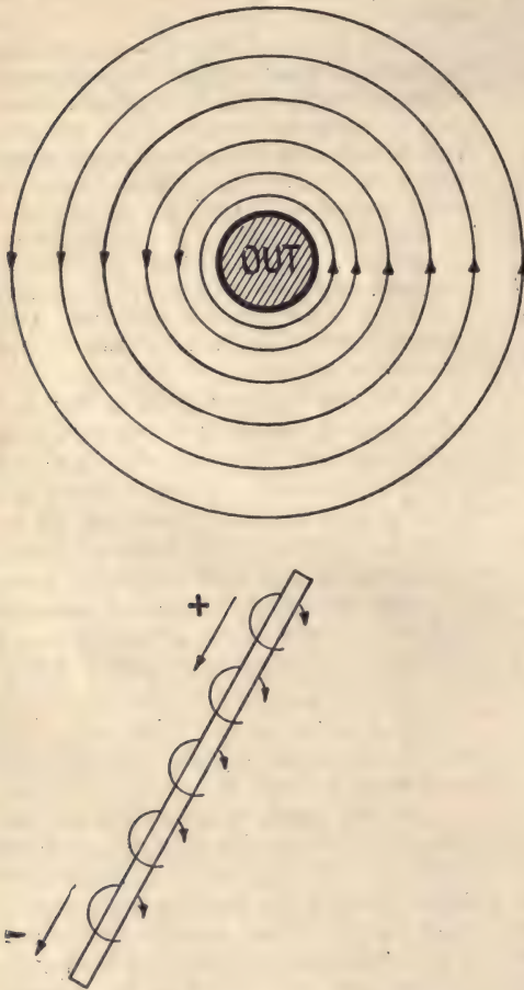
Fig. 12b—Showing Lines of Force Around a Conductor with Current Flowing Towards Reader.
