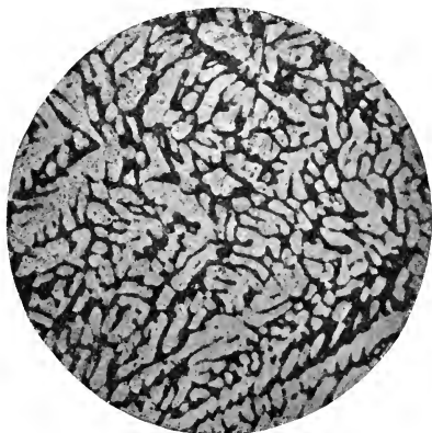
FIG. 7. — Gold, 31.5 per cent.; Cadmium, 68.5 per cent. \times 25 .
