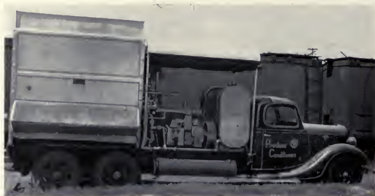
FIG. 2.—PORTABLE PRECOOLING PLANT MOUNTED ON TRUCK CHASSIS
