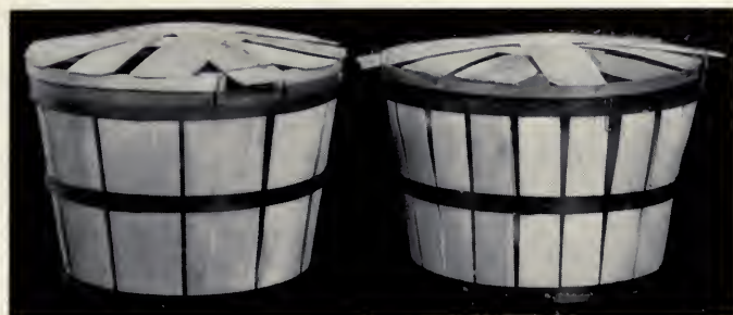
FIG. 4.—VENTILATED LEIGH TUB ( left ) AND VENTILATED TUB BUSHEL ( right ) USED IN TESTS
