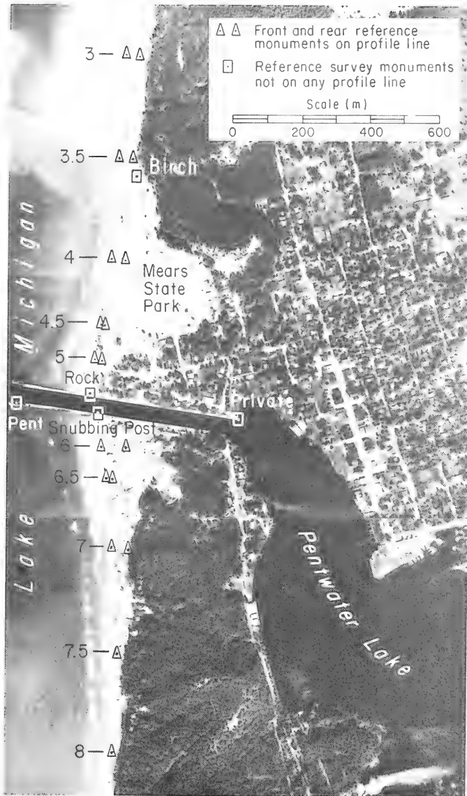
Figure 3. Profile stations in vicinity of Pentwater jetties.
