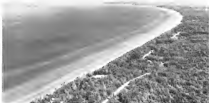
Figure 6. Longshore continuity of bars in the Great Lakes. The inner two to three bars are usually visible when viewed from high bluffs and dunes along the shore. In the above photo (taken about 900 meters above lake level) the inner three bars can be seen following the curve of the shoreline from station 10 toward Pentwater Harbor in the upper right corner (a distance of about 6 kilometers).
