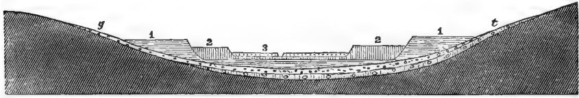
Fig. 12.—Diagrammatic Section of Postglacial and Recent River-gravels, etc. t , till ; g , glacial gravels ; 1, 2, 3, successive terraces of alluvial origin.
