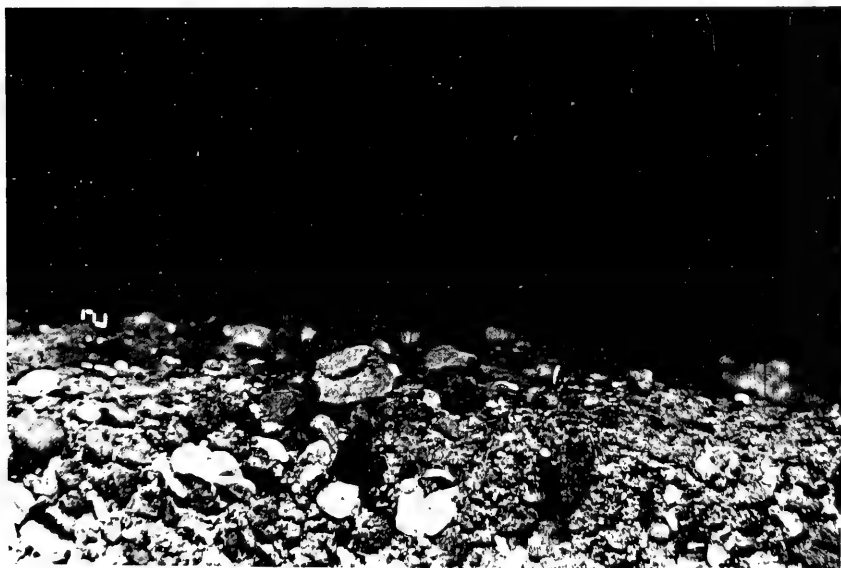
Figure 3-6. Two replicate REMOTS images from station E-6 near the apex of the historic disposal mound at the Brenton Reef site. The top image shows poorly-sorted medium sand (2 to 1 phi) exceeding the depth of prism penetration; the bottom image shows poorly-sorted granules (-1 to -2 phi). Scale of both images = 1X.
