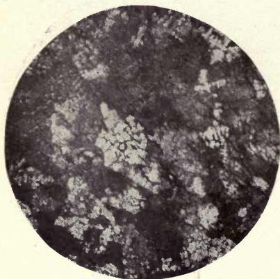
FIG. 18. ALLOY No. 5. x 40. 61.63% Cu, 38.25% Ni BY WEIGHT. ETCHED IN 1% FeCl 3 IN 1:1 HCl.
