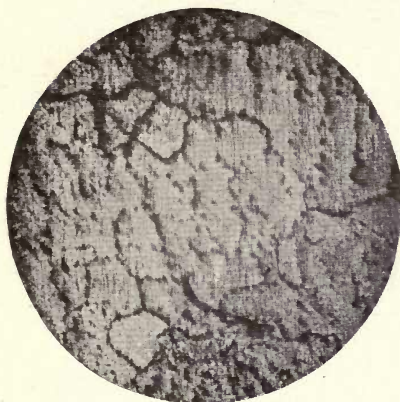
FIG. 22. ALLOY No. 9. x 40. 20.65% CU, 79.35% NI. ETCHED IN 1% FeCl 3 IN 1:1 HCl.
