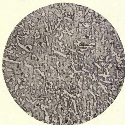
FIG. 64. ALLOY No. 55. x 40. APPROX. 56.6% Cr, 11.5% Cu, 31.9% Ni. ETCHED IN AQUA REGIA.
