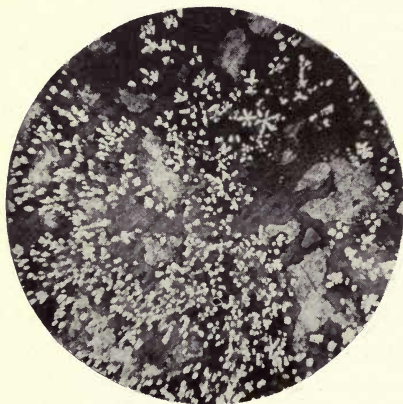
FIG. 52. ALLOY No. 39. x 40. APPROX. 35.29% CR, 64.71% CU.
