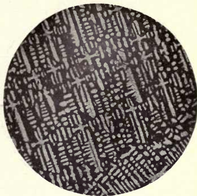
FIG. 39. ALLOYED No. 26. x 40. 19.30% CR, 44.08% CU, 36.34% NI. NOT ETCHED, BUT STAINED IN I IN KI.
