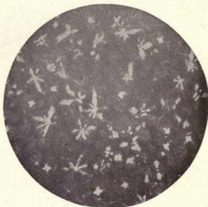
FIG. 27. ALLOY No. 14. x 40. 8.25% CR, 74.63% CU, 16.05% NI. ETCHED IN 1% FeCl 3 IN 1:1 HCl.
