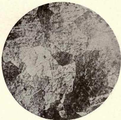
FIG. 43. ALLOY No. 30. x 40. 21.52% CR, 76.95% NI. ETCHED IN 1% FeCl 3 IN 1:1 HCl.
