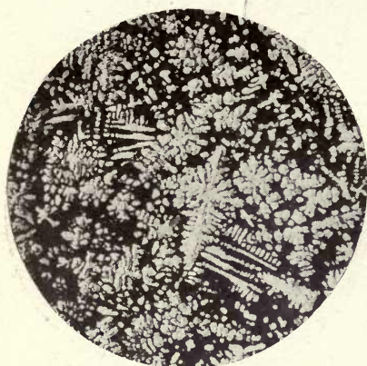
FIG. 54. ALLOY No. 41. x 40. 31.63% CR, 54.16% CU, 14.21% NI. STAINED IN I IN ALCOHOL.
