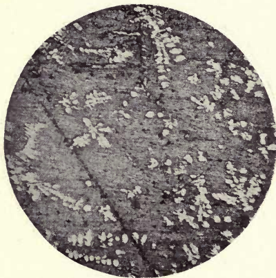
FIG. 44. ALLOY No. 31. x 40. 9.89% CR, 89.82% CU. NOT ETCHED. RELIEF POLISHING.
