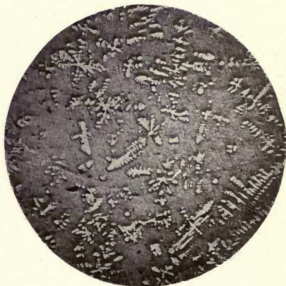
FIG. 53. ALLOY No. 40. x 40. 19.93% CR, 70.57% CU, 8.99% NI. NOT ETCHED. RELIEF POLISHING.
