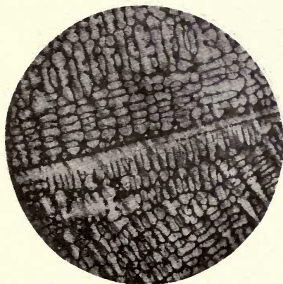
FIG. 48. ALLOY No. 35. x 40. 29.46% CR, 33.76% CU, 36.78% NI. ETCHED, THEN STAINED IN I IN KI.
