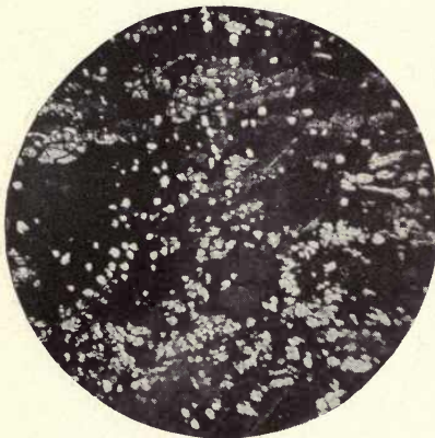
FIG. 36. ALLOY No. 23. x 40. 10.56% CR, 80.58% CU, 9.38% NI. ETCHED LIGHTLY IN 1% FeCl 3 IN 1:1 HCl.
