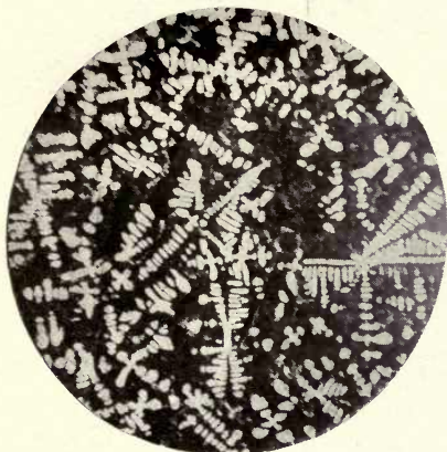
FIG. 39. ALLOYED No. 26. x 40. 19.30% CR, 44.08% CU, 36.34% NI. NOT ETCHED, BUT STAINED IN I IN KI.
