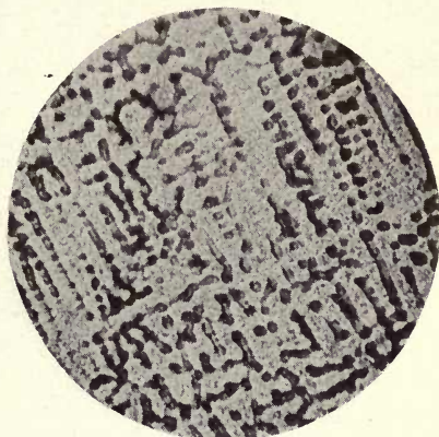
FIG. 31. ALLOY No. 18. x 40. 13.97% CR, 32.69% CU, 54.16% NI. ETCHED IN 1% FeCl 3 IN 1:1 HCl.
