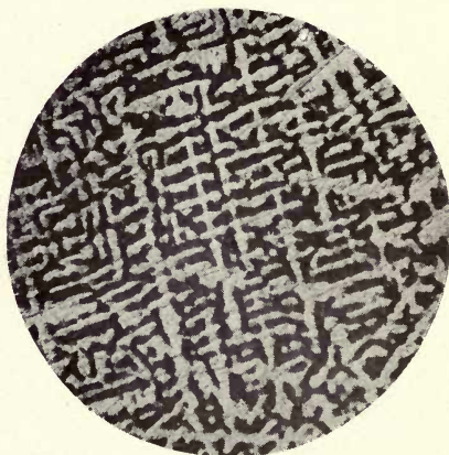
FIG. 29. ALLOY No. 16. x 40. 15.9% CR, 54.7% CU, 29.4% NI. ETCHED IN 1% FeCl 3 IN 1:1 HCl.
