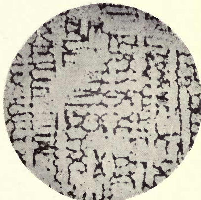
FIG. 49. ALLOY No. 36. x 40. 28.10% CR, 22.58% CU, 48.42% NI. ETCHED, THEN STAINED IN I IN KI.
