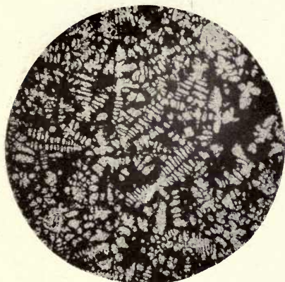
FIG. 46. ALLOY No. 33. x 40. 22.00% CR, 59.62% CU, 19.48% NI. ETCHED IN I IN KI.
