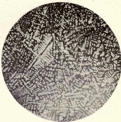
FIG. 19. ALLOY No. 6. x 40. 48.96% Cu, 49.90% Ni BY WEIGHT. ETCHED IN 1% FeCl 3 IN 1:1 HCl.
