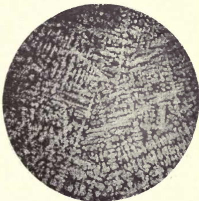
FIG. 17. ALLOY No. 4. x 40. 71.16% Cu, 28.46% Ni BY WEIGHT. ETCHED IN 1% FeCl 3 IN 1:1 HCl.
