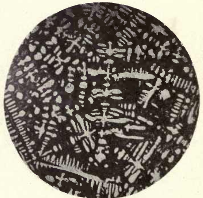
FIG. 37. ALLOY No. 24. x 40. 14.56% CR, 56.30% CU, 29.24% NI. ETCHED AND THEN STAINED IN I IN KI.
