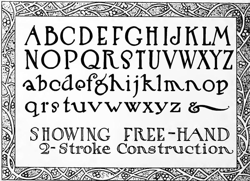
Original 15x21 inches, No. 2 pen showing 2 strokes joined on heavy portion of letters, air brush stipple back ground through stencil border, white strokes running through outlined with No. 5 pen.
