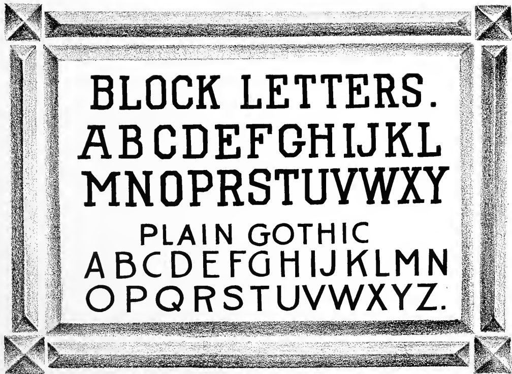
Original 10x14 stipple paper border, showing block and Egyption styles with No. 2 and 3 pens. Note square finish strokes. Pen held at right angles with paper, pointing straight at top of sheet.
