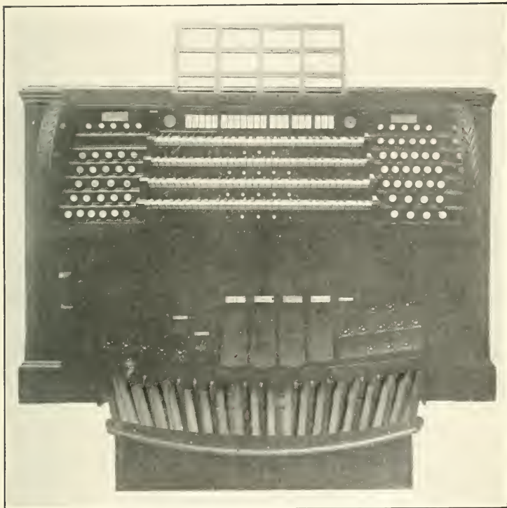
CONSOLE WITH STOPS ARRANGED IN TIERS; COUPLERS CONTROLLED BY TILTING TABLETS (M. P. Möller, Hagerstown, Md.)
