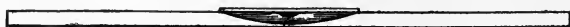
Longitudinal section of hollow-ground glass slide for observing bacteria in hanging drops.
