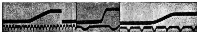
FIG. 120. String galvanometer records of the change of current obtained by opening the diaphragm in the rheonome (Fig. 119) at different rates. (K. LUCAS.)
