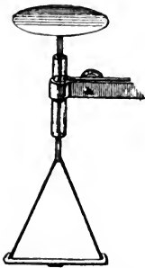
FIG. 428. Apparatus of von Kries for measuring capillary blood pressure.
