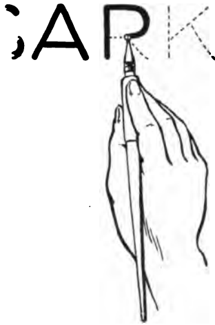
FIG. 23.—View from above of the correct writing position for pens of the flat shoe type.
