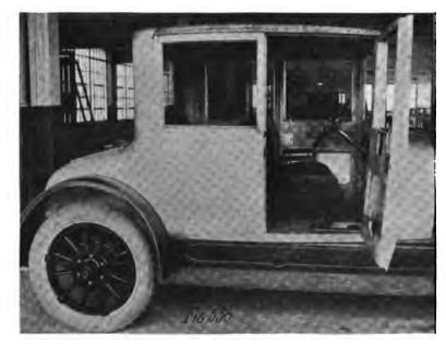
Four-passenger coupe in course of construction. Panels are all steel except the post covering, where aluminum is used. Composition roof, supported by slats
