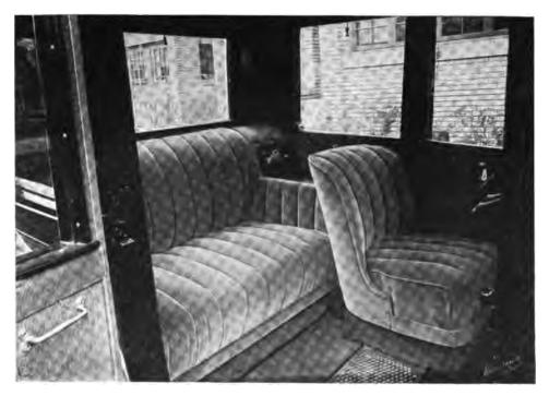
FIG. 491 A pleasing example of French plait upholstery in a gasoline car.
