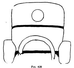
A large, round glass like this does not allow either the side passengers in the rear seat or the driver to see out of it.
