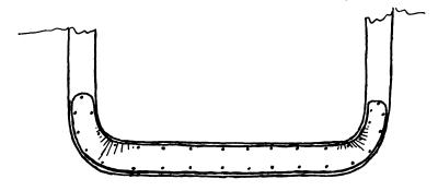
FIG. 196 . Cheapest design of sheet metal scuff plate
