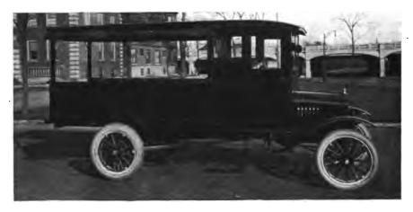
FIG. 570. Open express body, with enclosed cab for the driver
