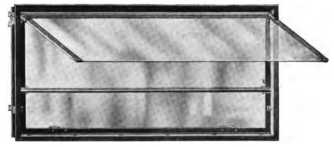
F1G. 372 A A type of "three-way" shield that is extensively used on large production as well as custom made cars. (Joseph N. Smith & Co., Detroit.)
