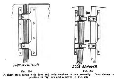
on the door, and which disengages the pin from the body section, permitting the door to be pulled right out. The door section is made of malleable iron and the pin on which it works is of steel, pressed into the iron. This door section sets on the side of the door frame, and it is bolted on, the bolts going right through the
