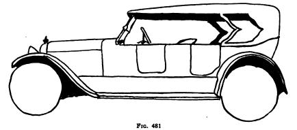
This top has comparatively straight lines with a solid side and an unusually elaborate side glass.
