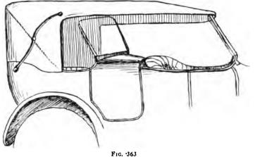
This shield rests on the end of a cowl-like cover, that fits across the opposite doors of the body. The cover and shield may be folded for ingress and egress. See Fig. 364.
