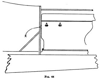
An example of interference between dash and engine
