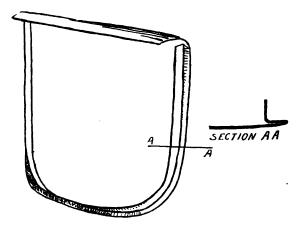
FIG. 188 The outer plate is bent down on to an angle and the angle provides the means of attachment to the door frame
