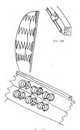
Fig. 507 If a unit spring construction is not used, each spring must fasten to the slat by staples, and they are tied together at the front with cords.
