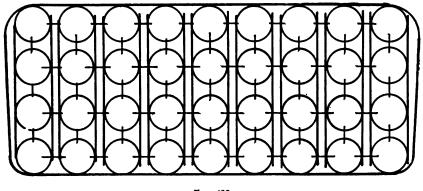
FIG. 499 A typical spring assembly with U-section metal base.
