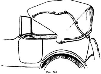
Single shield designed to protect rear seat passengers in a Victoria top body.
