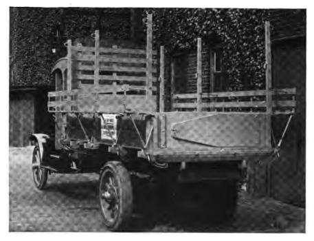
FIG. 602 "Everyway" body; sides at right angle to body, for carrying boxes and crates.
