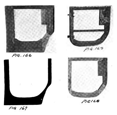
These four figures show the frame-up of a door, Figs. 168 and 169 picturing the completed frame.
