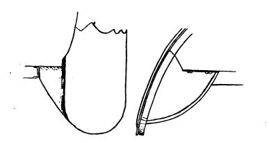
FIG. 318 One of the best ways to design a rear fender wing
