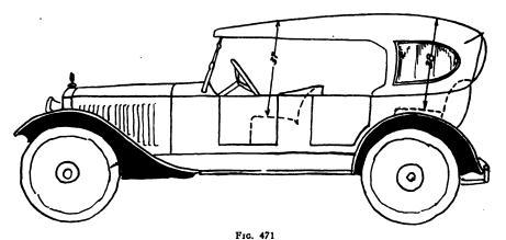
Typical five-passenger body with a California type top. This design gives ample head room.
