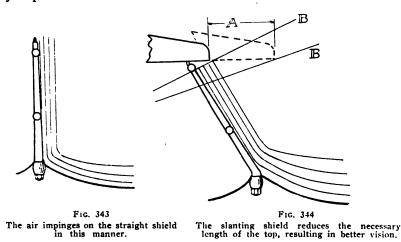
The desire to do away with the top straps that either extended to the front of the frame or attached to the cowl, resulted in the development of the side arm or "standard" type of shield. These standards were made high enough so that the
