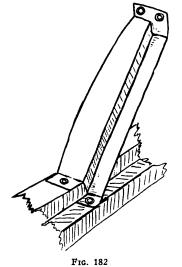
Toe block, riveted to the dash at the top and attached to the sills by wood screws
