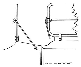
F1G. 342 One of the earliest types of windshields, fitted to brass or steel frames that clamped on the dash and were braced by long rods on the sides.
