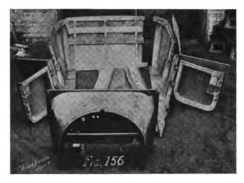
Front end view of body partially disassembled for shipping purposes
