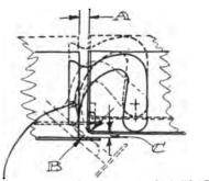
GROOVE FOR CLEARANCE AT CENTER OF THE DOOR. FIG. 219 Door post to illustrate the working clearance required
