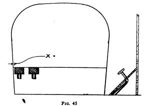
The toe boards are laid out to allow proper clutch and brake pedal movement
