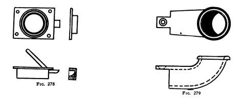
a great variety of different forms of bumpers devised. A number of designs have been developed that have springs in them to take up the shocks. There are some that have both springs and rubber, but the most satisfactory bumpers that have been devised are of rubber. The bumper design is affected by the door post construction in a similar manner to the strike. The first door condition would
