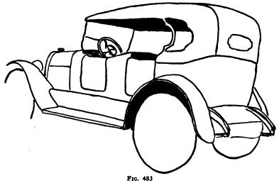
A rounded type of top with a fancy shaped side and side light. The back light is also rather ornate in design.
