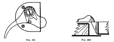
The lock shown in Figs. 241 and 242 is of a very simple construction, consisting of a base, a coiled spring, a stop plate and a handle.
