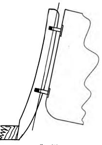
FIG. 212 Concealed type hinge swinging the door outward and slightly downward
