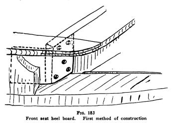
bodies for the doors. They attach to the door frames by suitable flanges. There are two methods of making these, in general use; the first and older method is specially adaptable to small quantities and its construction made is shown in the
