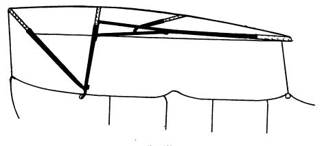
Fig. 377 Typical layout for bow sockets.
