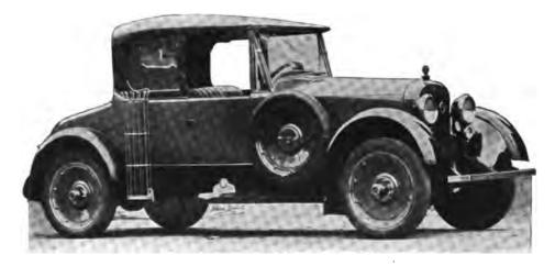
Fig. 470 A A California built car with top of striking design. This top is not built on to the car body, but with it, and is therefore stronger and more rigid than the usual California top. (Leach-Biliwell, Los Angeles, Calif.)
