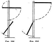
Showing the range of action with the joints located in different positions. It is obvious that the locations shown in the right hand figure are the better.
