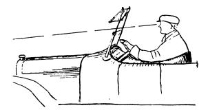
FIG. 346 The double shield can be closed in bad weather and in good weather opened at the top, while the lower portion deflects the air.
