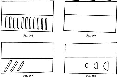
In Figs. 105 to 108 are shown four different styles of ventilating slits or "louvres," as they are properly termed
