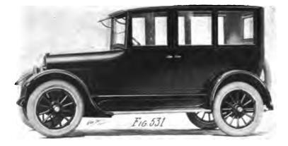
A seven-passenger car manufactured on a large scale. Six-cylinder chassis, 124-inch wheelbase
