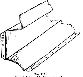
Typical design of heel board or raiser
