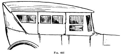
Back curtain with extensions running to the back how sockets. These are called "gypsy" curtains.
