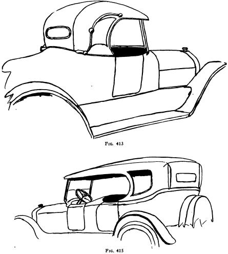
The light with the rounded end like that shown in Fig. 413, and the rectangular light shown in Fig. 415, are good, conservative shapes for the curtain maker to carry in stock. They can be worked into practically any design.
