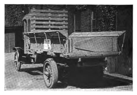
Fig. 601 "Everyway" body with sides let down at an angle, for carrying sacks and bales.
