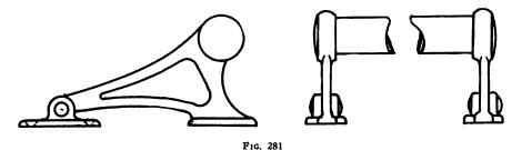
A conventional design of foot rest with nickel plated rod and nickeled or enameled end brackets
