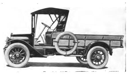
FIG. 555. Example of open express body with top over seat
