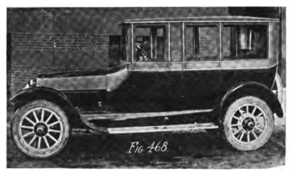
A detachable top assembled on a car body, ready for painting. The glasses in the doors are constructed so that the upper half can be lowered when desired.
