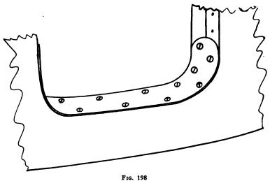
Scuff plate of polished aluminum, attached by French licad wood screws
