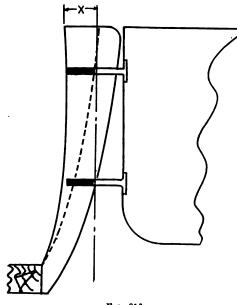
FIG. 213 Concealed hinge on heavier pillar, swinging the door square
