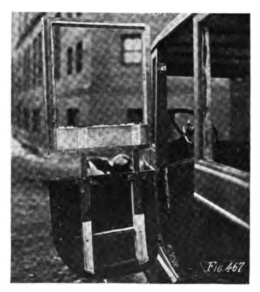
The upper sections of the doors on the detachable top are attached to the regular car door as shown in this photograph.
