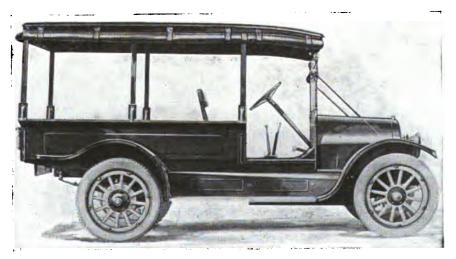
FIG. 557. Typical light delivery or package body, with flare boards and curtains at side and rear
