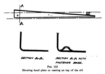
under the hood; this is to prevent squeaking as the hood works back and forth when the car is in service.
