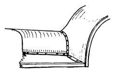
FIG. 336 The older method was to bolt the side apron on to the running board. A half-oval moulding was welded to the side apron and this was countersunk for French head bolts.
