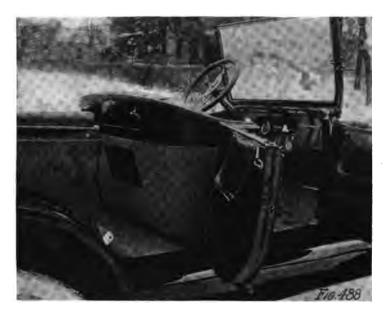
Example of rear compartment or tonneau trimming, showing door and back of front seat.
