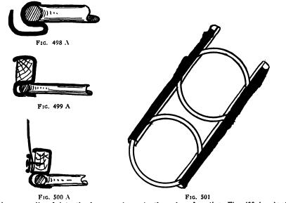
The springs are clipped into the base as shown in the enlarged section, Fig. 498-A. Another method is to have a section like that shown in Fig. 499-A. The cushion cover is held on the spring by tacking the lower edges, as in Fig. 500-A. The outer spring clips to the inner edges of these bases, the other springs are held in place by V-strips as shown in Fig. 501.
