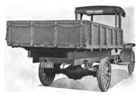
FIG. 592. Express Type Sides fitted to a heavy truck for hauling sand and gravel
