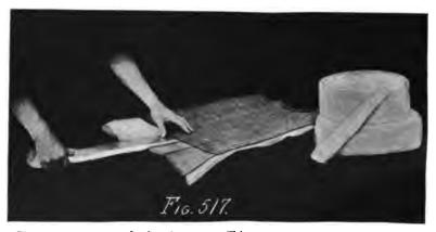
The cotton comes ready for the pipes. This cut shows the cotton and the method of inserting it into the pipes.
