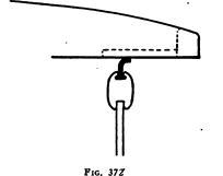
A weather strip is often fitted in between the top of the windshield and the car top. A close joint should be made the entire length of the rubber strip.
