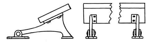
FIG. 282 Foot rest made of two end brackets and a center board, covered with a suitable material
