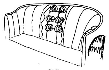
FIG. 513 In order to economize in the use of hair, several constructions have been developed, one of which is shown here. Another construction is illustrated in Fig. 512.
