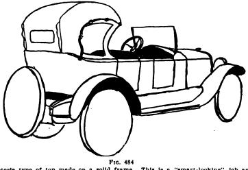
Victoria type of top made on a solid frame. This is a "smart-looking" job and can be built more easily than a regular Victoria top.
