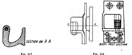
FIG. 217 Illustrating further the construction of a type of concealed hinge. See also Fig. 216 on page 105.
