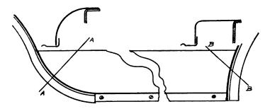
FIG. 337 A cheap method of assembling a side apron to a car, which does not protect the running boards from the mud which works in between them and the fender.
