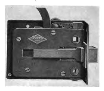
FIG. 249 This lock can be locked from the inside by turning the knob, or locked from the outside by the cylinder lock, which operates the same pawl as the knob does (Ferro-Stamping & Mfg. Co, Detroit)
