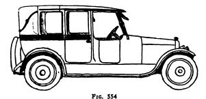
This sketch represents the same body as the one shown in Fig. 553 above, but with the rear closed, fully protecting the passengers in the worst weather
