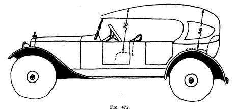
Same body as shown in Fig. 471, but with a top of more "funcy" style. The rounded back cuts down the rear seat head room to about 36 inches on the rear seat. The rounded front also reduces the front seat head room to the same number of inches.
