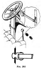
Device placed on door to hold it slightly open for ventilation
