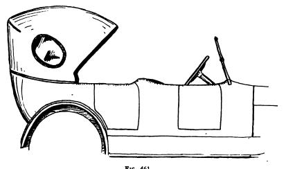
Fig. 461 A solid construction, eliminating the joint iron. This top cannot be folded.
