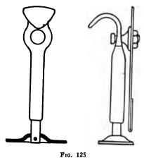
Fastener hooking on to a stud
