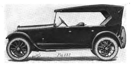
FIG. 137 A 1922 Buick body with low cut sides
