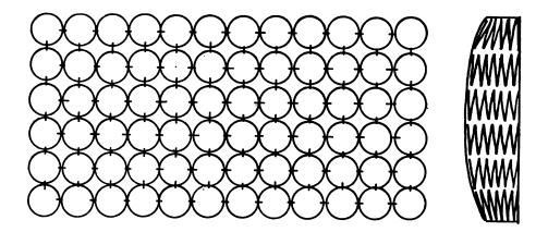
FIG. 508 The modern type of cylindrical-shaped spring has to be spaced close together to give proper supporting surface for the hair.
