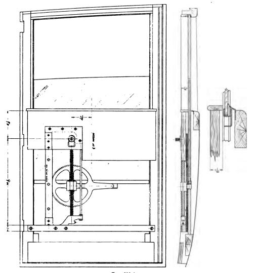
FIG. 309 A Reproduction of factory blue print, showing construction and method of installing the Jos. N. Smith & Co. window regulator
