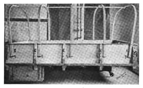
Fig. 598 <sup>4</sup> An American army truck body, "knock-down" construction.
