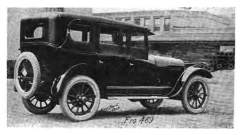
A California top, designed on good lines and furnished with side curtains. No framework is visible around the glass lights. The covering material is leather substitute in a color to harmonize with the car painting.
