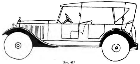
In an ordinary folding top the sides of the back curtains are generally extended to make what is termed a "gypsy" curtain.
