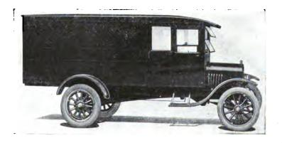
FIG. 569. Figs. 568 and 569—Full panelled bodies are used on speed wagons. Fig. 568 has driver's seat protected by side curtains, while Fig. 569 shows the driver's seat fully enclosed
