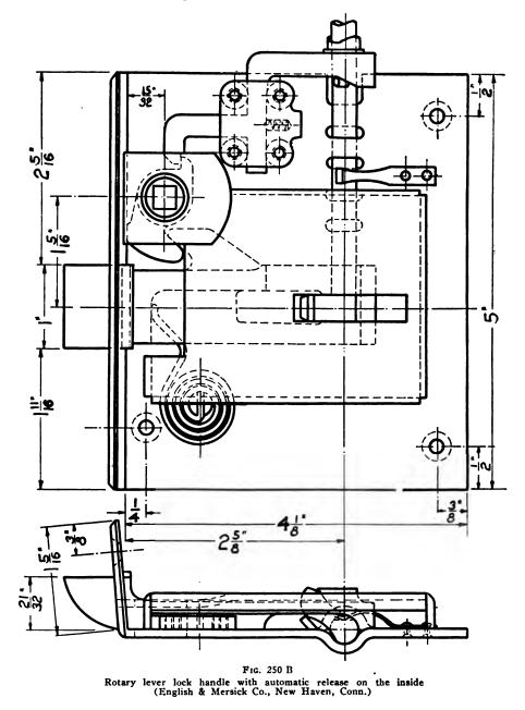
from the inside by turning the knurled knob or locked from the outside by the cylinder lock which operates the same locking pawl as the knob does. The illus-
