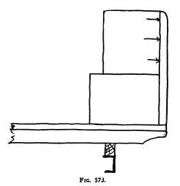
Side strains often exert a leverage by being imposed against the stakes, as shown here
