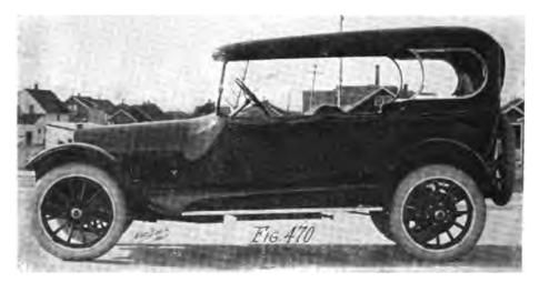
California top with metal frame glasses. Window glass is usually beveled-edge plate and is furnished assembled in the frames ready to use by several manufacturers.
