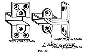
A hinge that has the same door section as that shown in Fig. 220, but the body section is made so that when the two screws at A are taken out in the upper and lower sections, the door can be removed
