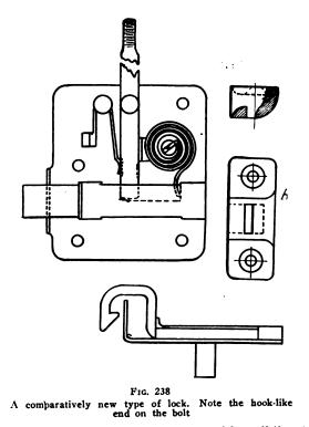
will be seen that it consists of a body or base plate with a sliding bolt operated by a pivoted lever. Two springs are used, one to throw the bolt out and the other to keep the lever stationary while the bolts work in upon striking the door post. It will be
