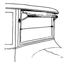
FIG. 304 This sunshade has hinged brackets and the cloth is attached to a spring roller. A slight jerk releases the catch and the shade folds up when not needed.
