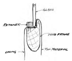
Fig. 431 Method of installing light with wood frame is shown in this diagram.
