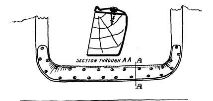
FIG. 200 One of the best designs for a scuff plate, with section through AA.
