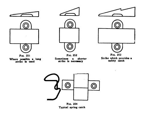
door closes, the lock bolt has to be thrust back, and in order to do this easily a suitable bevel is provided that will make a sliding contact. The length of the sliding face of the strike is governed by the thickness of the door frame and lock pillar. When it is possible, a long strike like that shown in Fig. 251 is used, but
