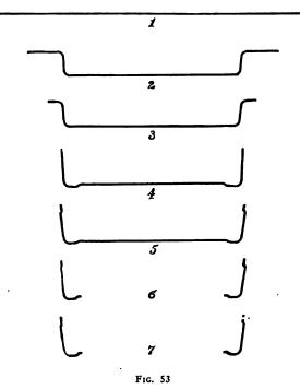
Difference in the shape of a shell after each of seven operations
