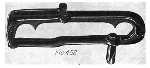
This holder has an extension on it, cut at an angle as shown, so that by tightening the cap screw it will be held very securely.
