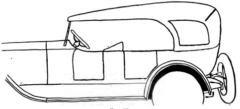
FIG. 475 California top fitted to a low sided body.
