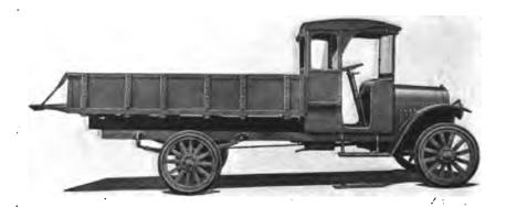
FIG. 584. Platform with sides added
