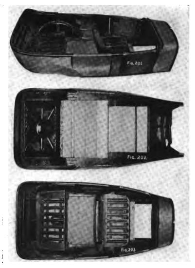
FIGS. 201, 202, 203 Example of all steel body construction (Edward G. Budd & Co., Philadelphia, Pa.) Shows different views of same body so that the construction can be easily seen.
