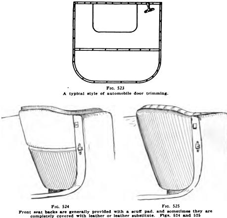
Front seat backs are generally provided with a scuff pad, and sometimes they are completely covered with leather or leather substitute. Figs. 524 and 525 show examples of these two methods.
