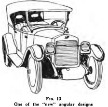
The angular type of designs which are shown in Figs. 13 and 14 are "new" designs, the predominating feature being a decided tendency to flat surfaces and sharp corners. In Fig. 13 it will be seen that the radiator has sharp corners at
