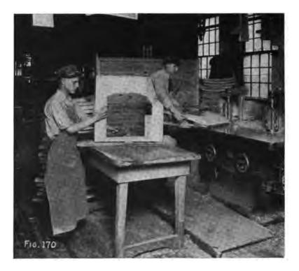
The door is shaped on its outer edges in a form
