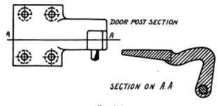
FIG. 216 Illustrating construction of a type of concealed hinge
