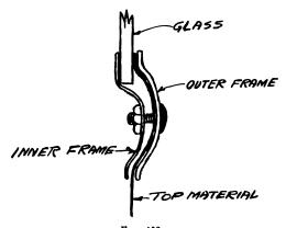
Fig. 430 Diagram showing method of installing Brewer-Titchener style of light.
