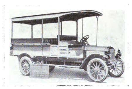
FIG. 567. Another speed wagon, with stationary posts and canopy top
