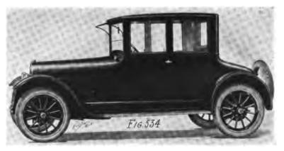
Coupé body on four-cylinder chassis, 109-inch wheelbase.
