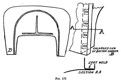
Shape of a typical shroud in the condition in which it comes off the dies and before final operations are made on it
