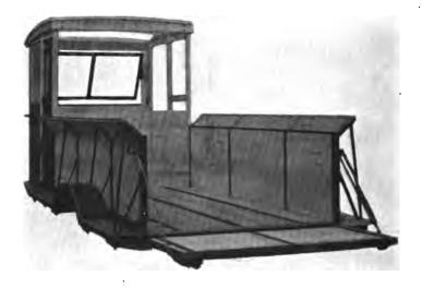
FIG. 622 Open express body with cab attached. The outer side extends beyond the body to make a running board and fender. The brace system insures very strong side panels, and the body width is the same as the cab.
