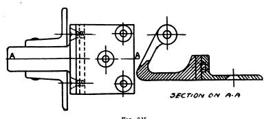
FIG. 225 Hinge made of malleable iron. The door is removed by taking out two screws in each door section
