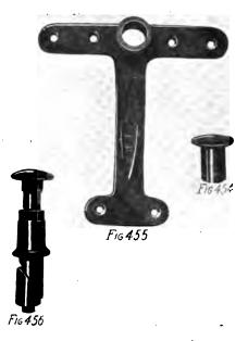
Fig. 454 is a cap used to plug the hole: Fig. 455 is a new style front top iron; Fig. 456 detachable top iron stud The Victoria top is quite popular on cars for use in the city, as it has a striking appearance and is very adaptable for city use. The construction is identical to those tops that were used on carriages. The general form of construction is
