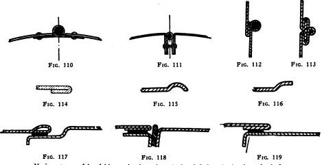
Various types of hood hinges, beads and methods of fitting the hood to the body
