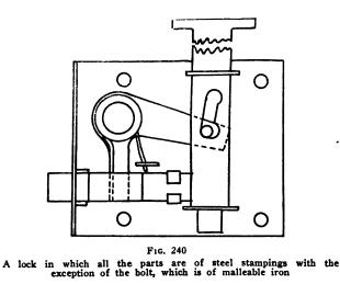
This method of operating a lock is preferred by some, and there are also movements worked out to operate the bolt by pulling up or pushing down, but these actions are not as popular as the standard sideways action of the door lock shown in Fig. 229.
