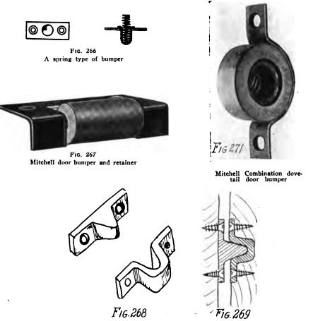
Typical design of dovetail, and cross-section of same, taken through the door post, dovetail and door frame.
