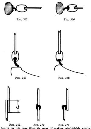
The seven figures on this page illustrate ways of making windshields weatherproof by means of fillers, usually of rubber, between the glass frames and the standards.
