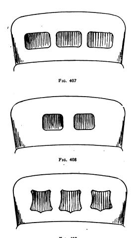
Fig. 409 These three drawings and the ones on page 188, show different shapes and arrangements of back curtain lights.
