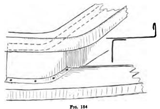
Front seat heel board. Second method of construction
