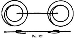
The centers of the springs are tied together with wire or clips similar to the manner shown in this diagram.
