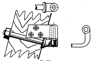
FIG. 215 Similar in construction to Fig. 214, but the two parts, instead of being riveted, contact on one face.
