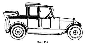
The landaulet is a closed car along the same lines as a limousine, but the rear part of body can be folded back. Sketch shows rear opened up
