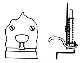
. Fig. 126 Concealed type of fastener in which only the handle is visible from the outside
