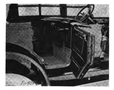
Another method of treating the door and back of front seat in a touring car or "phaeton."
