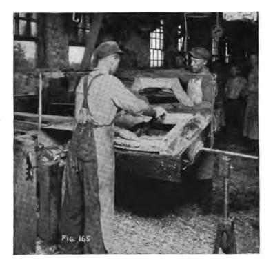
The door frame is securely clamped in a heavy frame that slides on irregularly shaped guides that give the desired sweeps while the wood is being machined.
