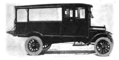
Fig. 621Canopy top body using same parts as in Fig. 620, only the roof is replaced by the extension of the canopy top.
