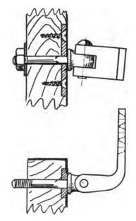
FIG. 214 Knuckle type hinge. With this style hinge the door is not readily removed
