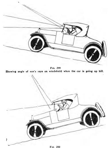
Showing angle of sun's rays on windshield when the car is going down hill.
