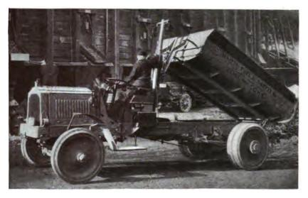
$$\rm Fig.~604$$  Contractors' dump body with mechanical hoist using engine's power.
