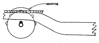
F1G. 47 A special housing at rear of body to clear the rear axle housing
