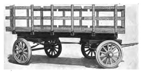
FIG. 610 Truck trailer of the platform type with side stakes.
