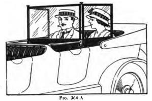
A standard, patented type of rear windshield. (Tonneau Shield Co., New York City.)
