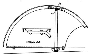
F1G. 325 This fender has a larger and longer wing that extends down to the frame and is secured by a bracket
