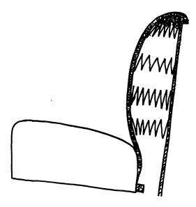
FIG. 511 A sectional view of a trimmed back.
