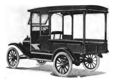
F1G. 558. Four-post light delivery body with flare boards and curtains side and rear
