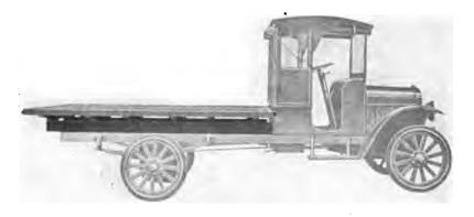
FIG. 571. Truck with driver's seat and cab, with a typical platform mounted in the rear
