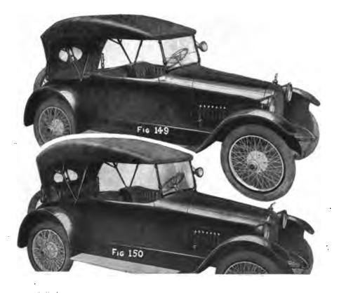
Another type of convertible Roadster is shown in Figs. 149 and 150. Fig. 149 shows the top up and rear compartment closed. In Fig. 150 the top is shown up, and the seat back raised to provide two extra seats.
