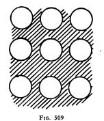
Cloth laid upon double cone springs showing area in shaded lines where there is no support on spring.
