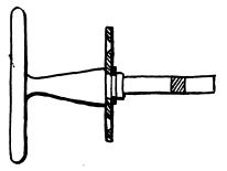
FIG. 244 Construction of a typical door handle
