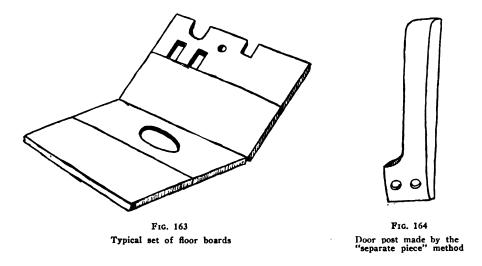
also muffler cut-out pedal. A typical set of floor boards is shown in Fig. 163. The front door post is made of ash, elm or maple, and is shaped on the outside to give the desired sweep to the body, and on the inside for the correct flare for the door.
