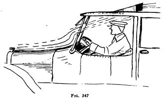
Under this condition there should be a ventilator in the top or an open window in the rear to avoid unpleasant air currents.
