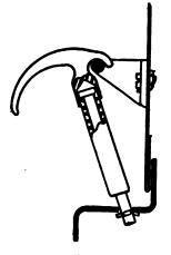
FIG. 124 Fastener hooking on to a bracket
