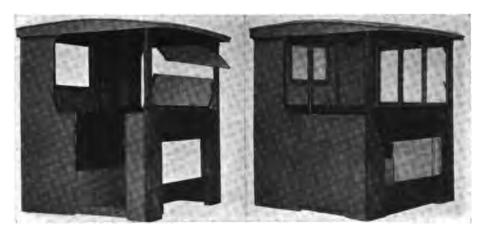
FIG. 623 Sliding door cab showing the cab wide open on the left and closed on the right. (Highland Body Mfg. Co., Cincinnati, Ohio.)
