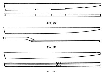
Fic. 174 Various forms of Sills. Fig. 172, Flat Sill; Fig. 173, Upset Sill; Fig. 174, Built-up Sill
