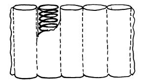
FIG. 498 The "Marshall" type springs are each enclosed in a cotton cylinder, the springs being packed closely together.
