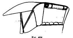
Three piece back curtain, permitting center section being rolled up in warm weather.
