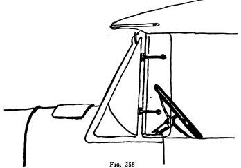
This car has the triangular side glass frames on each side of the windshield, and an adjustable extension to deflect air currents away from the interior of the body.
