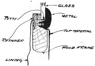
Fig. 429 Diagram showing method of installing Johnston type of light.
