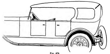
FIG. 476  $F_{\rm Here, the body sides are higher than in Fig. 475, consequently we get better balance in the design.$
