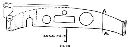
Construction of reinforcement plate for steering column bracket
