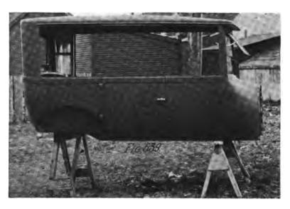
Same job as above with all the posts removed so it can be seen how "open" the body can be made when desired.
