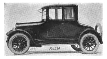
Typical four-passenger car, made in quantities. This body is on a six-cylinder chassis, 124-inch wheelbase.
