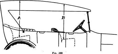
Method of determining head clearance in designing an automobile top.
