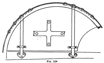
Here the fender wing is short and is secured to the irons by small straps of steel
