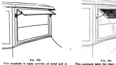
This sunshade is made entirely of metal and is adjustable to a small degree.
