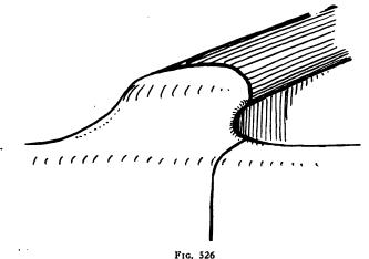
Top trimming on the front seat that has the double cowl. The leather in this case is stretched tightly over the wood center rail.
