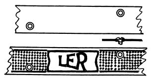
FIG. 199 Scuff plate of aluminum with etched design or car name
