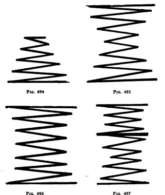
FIG. 496 FIG. 497 In Figs. 494 to 496 are illustrated the shapes of the cushion springs referred to on page 225. In Fig. 497, is shown a section through a typical "double-deck" spring construction.
