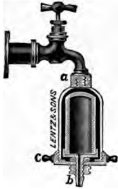
FIG. 26.—Domestic filter—Berkefeld: a , point of attachment to faucet; b , outlet.
