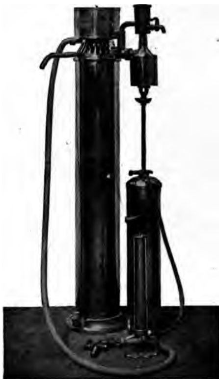
FIG. 55.—Forbes' portable water sterilizer, army type.
