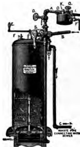
FIG. 25.—Mechanical filter: A, inlet pipe; B, outlet pipe; C, waste pipe; D, valve to cut off water from filter; E, lever to operate the agitator; F, air valve; H, handle of valve used to change the course of the water through the filter; I, distal attachment of coagulating tank to inlet pipe; K, lever valve regulating the quantity of alum supplied; O, proximal attachment of coagulating tank to inlet pipe; P, waste pipe leading from the coagulating tank to the sewer; Q, valve which fastens on the cover of the coagulating tank; S, pointer which indicates the course of the water through the filter; T, sight glass.
