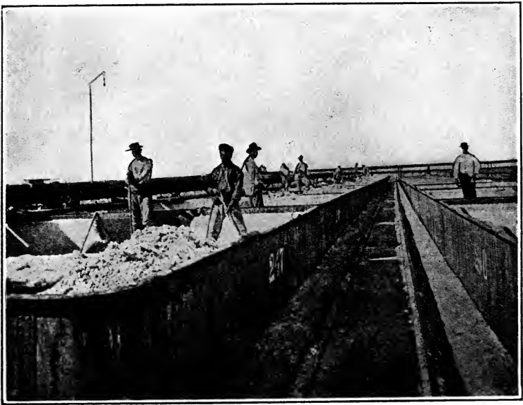
Fig. 71.—Crystallizing pans with nitrate of soda.
