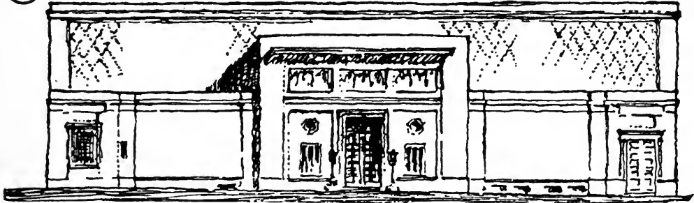
FIG. 139.—The New York State Education Building, Albany, by Palmer and Hornbostel. Here the façade takes the form of a screen behind which occurs the fenestration required for the various divisions of the plan. Expression of individual apartments is subordinated to the dominating idea of a highly monumental effect. FIG. 140.—Design for an Art Gallery by Easton and Robertson. Normal fenestration is here not desired, and the elevation expresses the requirements of the art gallery plan type.
