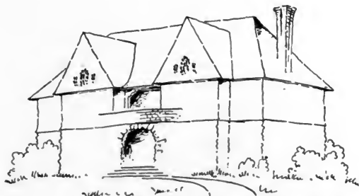
253. Ridge of link raised above those of members; the latter becoming subordinate masses upon a single main mass.
