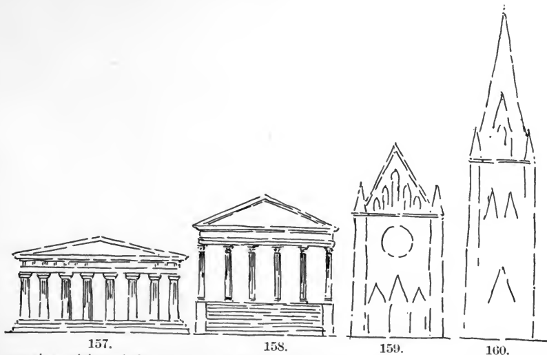
157. 158. 159. 160. Progressive raising of the lines of the gable with the lengthening upward of the front.
