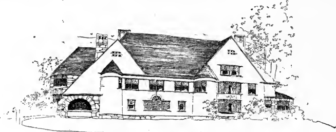
255. Double unsymmetrical group of gables, with an additional double symmetrical group of turrets.
