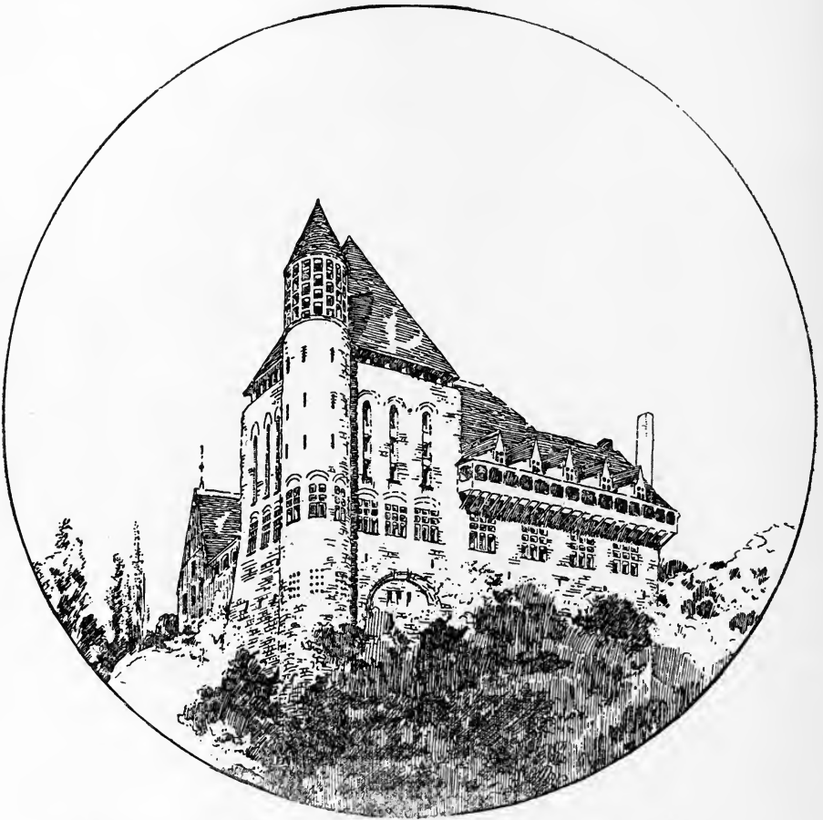
134. Design for Soldiers' Home, Minneapolis, Minn. Grouping of windows. Triplet windows in mass. Four windows in appendage.
