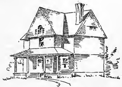
250. Same as 249. Ridge of subordinate gable raised to level of main ridge. A faulty composition.
