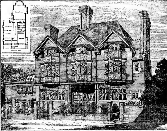
70. Residence, Frank Hall, Hampstead, London. An example of three equal subordinate gables.
