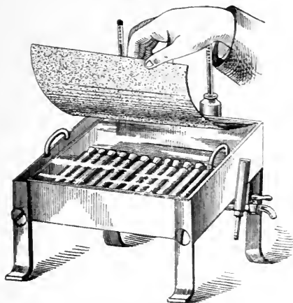
Chamber for sterilizing and solidifying blood-serum. (Кочн.)
