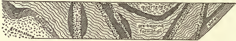
FIG. 142.—Generalized section in Marquette district, Michigan, showing relations of all classes of ore deposits to associated formations. On the right is soft ore resting in a V-shaped trough between the Siamo slate and a dike of soapstone. In the lower central part of the figure the more common relations of soft ore to vertical and inclined dikes cutting the jasper are shown. The ore may rest upon an inclined dike, between two inclined dikes, and upon the upper of the two, or be on both sides of a nearly vertical dike. In the upper central part of the figure are seen the relations of the hard ore to the Negaunee formation and the Goodrich quartzite. At the left is soft ore resting in a trough of soapstone which grades downward into greenstone. (After Van Hise, Bayley and Smyth, U. S. Geol. Survey. )
