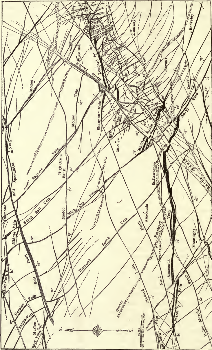
FIG. 156.—Horizontal section of part of Butte district, Montana, 4600 feet above sea level (about 1500 feet below the surface). (After Sales.)
