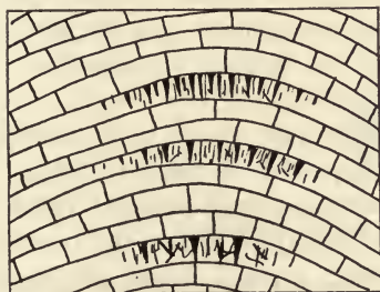
FIG. 79.—Diagram showing brittle beds fractured at and near the axis of an anticline.
