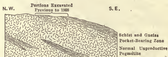
FIG. 12.—Sketch of pegmatite with zone of tourmaline pockets near the top of Mount Mica, Paris, Maine. (After Bastin, U. S. Geol. Survey. )
