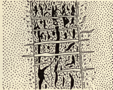
Legend for Fig. 83: — Quartz ··· Quartzite * Sulphides, chiefly galena S Siderite ■ Quartzite, partly replaced by siderite Scale: 0 1 2 feet
