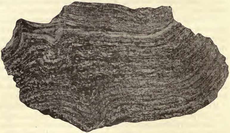
FIG. 58.—Polished surface of schistose ore metamorphosed by pressure, Milan mine, New Hampshire.
