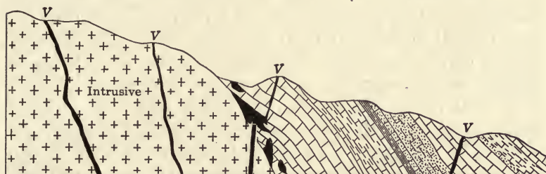
FIG. 19.—Section showing sedimentary rocks intruded by igneous rock, with contact-metamorphic deposits (irregular black areas) and veins.
