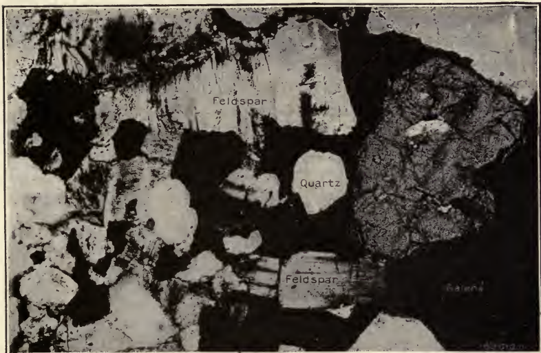
FIG. 9.—Section of ore formed by magmatic segregation. Well-shaped crystals of feldspar and quartz, partly dissolved are floated in a matrix of galena.
