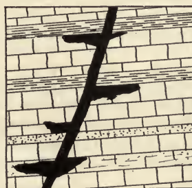
FIG. 5.—Replacement vein filling a fissure and replacing wall rock along the fissure.
