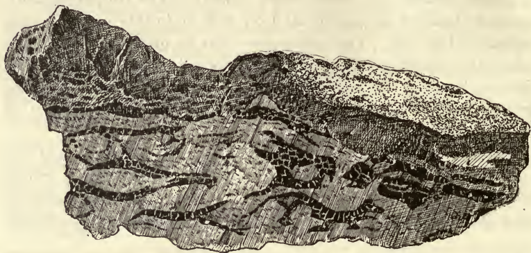
FIG. 32.—Section of chalcocite (light) replacing coal (dark) Nacimiento district, New Mexico. Upper part of specimen is altered by oxidation. (Redrawn from plate by Lindgren, Graton, and Gordon, U. S. Geol. Survey.)
