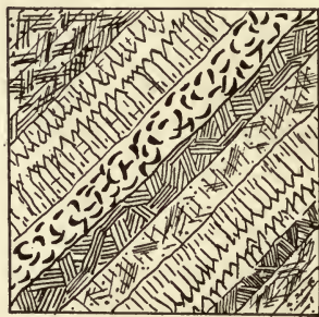
FIG. 2.—Section of vein with crustified banding.
