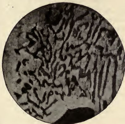
FIG. 71.—Graphic intergrowth (primary) of chalcocite (light) and bornite (dark), Wall mine, Virgilina district, Virginia and North Carolina. (After Laney.)
