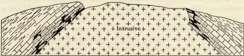
FIG. 17.—Diagram showing relations of contact-metamorphic deposits (black) to contact metamorphic zone (stippled) and to intrusive mass.
