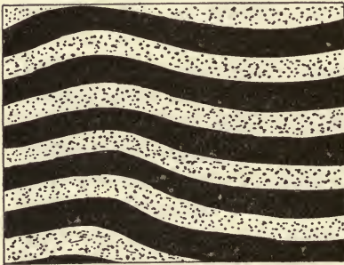
FIG. 38.—Banded ore of sedimentary origin, Kennedy mine, Cuyuna range, Minnesota. Chert (light) alternating with hematite (black). (About natural size.)
