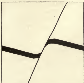
FIG. 51.—Vein curved near fault.
