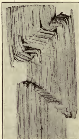
FIG. 78.—Column of oak deformed by applying pressure in direction of arrows. (After Lang.)
