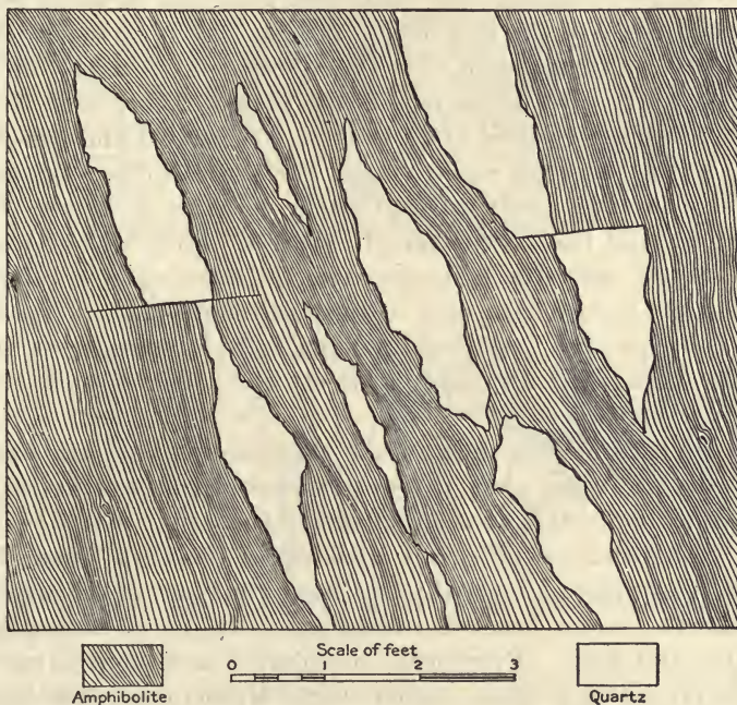
FIG. 23.—Vertical section in Schlegelmilch mine, York County, South Carolina, showing lenticular bodies of quartz in amphibolite schist. (After Graton, U. S. Geol. Survey. )
