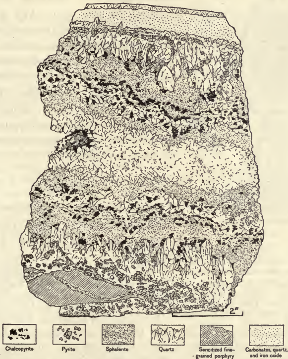
FIG. 27.—Section of banded vein, Pinos Altos district, New Mexico. (After Paige, U. S. Geol. Survey.)
