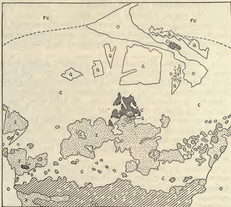
FIG. 20b.—Key to Fig. 20a. Fc , Fine-grained calcite of normal limestone, with dotted line indicating approximate transition to coarse calcite; C , coarse-grained calcite; Q , quartz; S , sericite; G , garnet; Z , zinc blende; Cu , chalcopryrite; O , open field. (After Lindgren, U. S. Geol. Survey .)
