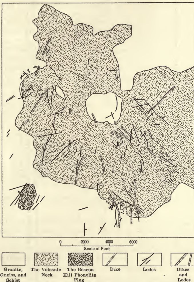
FIG. 108.—Plan of the principal fissures of the Cripple Creek district, Colorado on plane 9,500 feet above the sea. (Based on map by Lindgren and Ransome, U. S. Geol. Survey.)
