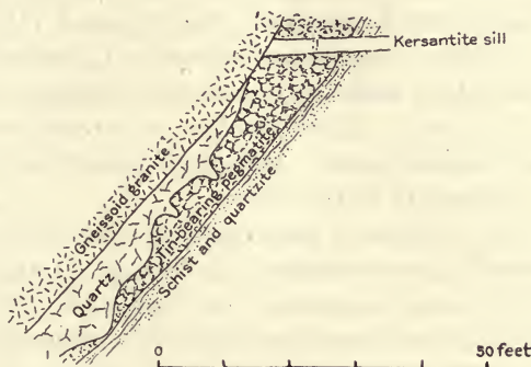
FIG. 205.—Section of tin deposit at Silver Hill, near Spokane, Washington. (After Collier, U. S. Geol. Survey .)
