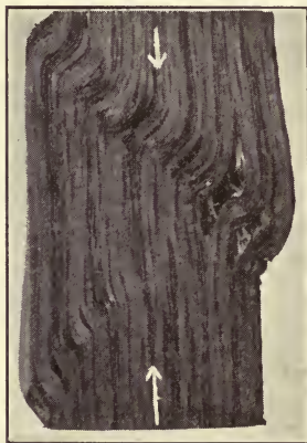
FIG. 77.—Block of oak deformed by applying pressure in direction of arrows. (After Lang.)
