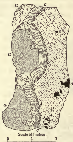
FIG. 28.—Sketch of specimen showing cementation of fragments of galena ( a ) belonging to the first period of deposition by a crustified material belonging to the second period and deposited in the following order: 1, Finely banded (crustified) brown carbonates ( b ); 2, a thin crust of quartz with sulphides ( c ); 3, mingled brown carbonates and fine quartz ( d ) containing some pyrite ( e ) and a little galena ( a ). (After Spurr, Garrey, and Ball, U. S. Geol. Survey .)
