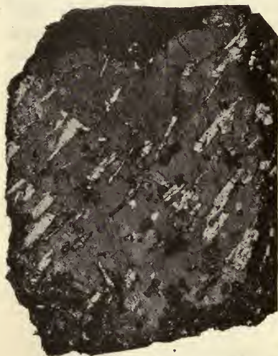
FIG. 8.—Iron ore formed by magmatic segregation, from Iron Lake, Minnesota. Dark is intergrowth of magnetite and ilmenite; light is feldspar. (After Singewald.)
