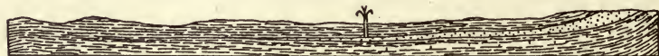
FIG. 210.—Diagram illustrating the thinning out of a porous bed between two impervious beds. (After T. C. Chamberlin, U. S. Geol. Survey. )
