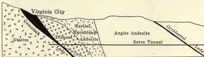
FIG. 191.—Section through Comstock lode, Nevada, on Sutro tunnel. Black is quartz and vein matter. (After Becker, U. S. Geol. Survey.)
