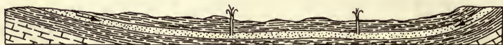
FIG. 209.—Diagram illustrating chief requisite conditions of artesian wells. (After T. C. Chamberlin, U. S. Geol. Survey. )
