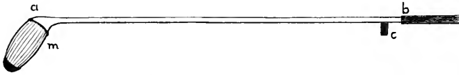
FIG. 390. Diagram of Marey's cardiac 'sound,' consisting of a long tube ab , terminating at one end in the ampulla m , which is covered with an elastic membrane. The side-piece c serves to indicate the position of the ampulla after it has been introduced into the vessels.
