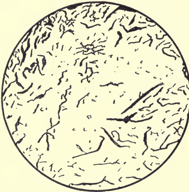
FIG. 2.—Pen sketch of graphite in field of comparatively pure iron.
