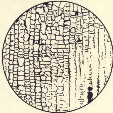
FIG. 4.—Pen sketch of iron crystallization with network of iron sulphide. Sulphur 4.2 per cent. (Stead.)
