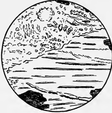
FIG. 1.—Pen sketch of needle and irregular shaped cementite in relief, in white field of austenite.
