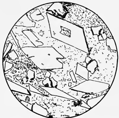
FIG. 6.—Pen sketch of iron with 11.07 per cent. phosphorus, showing rhombic crystals of iron phosphide in ground mass of solid solution of iron phosphide in iron. (Stead.)
