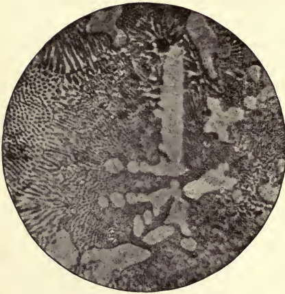
FIG. 26. — Silver-copper alloy. Showing "eutectic" and silver dendrites.
