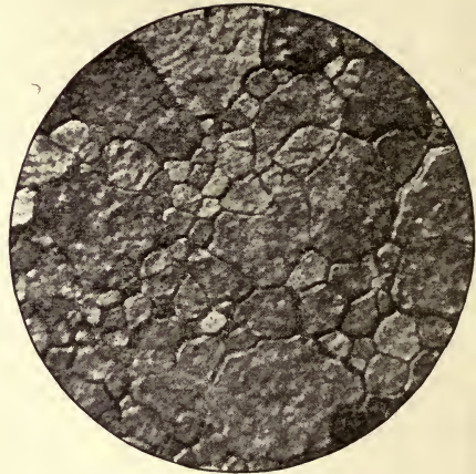
FIG. 26a. — Microstructure of tin. Showing crystal outlines.
