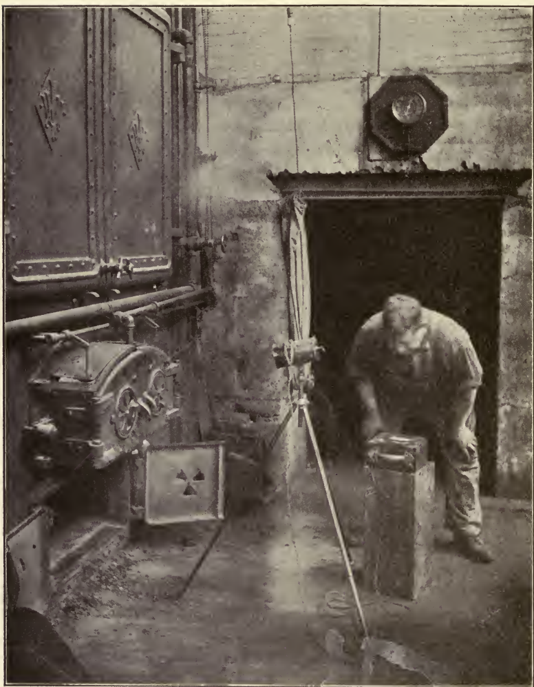
FIG. 61. — Féry pyrometer set up for an observation.
