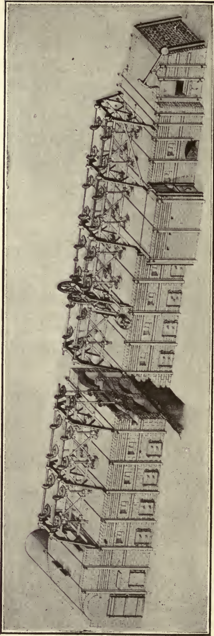
FIG. 161. — General view, Edwards duplex roasting furnace.
