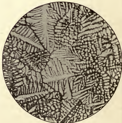
FIG. 26c. — Aluminium cast on stone. Showing crystal structure.
