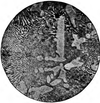
FIG. 26. — Silver-copper alloy. Showing "eutectic" and silver dendrites.
