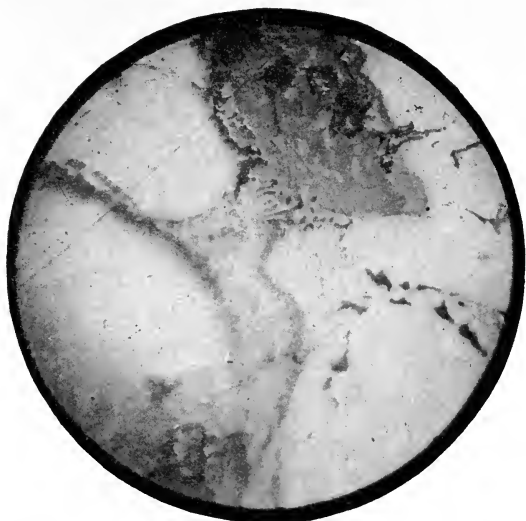
FIG. 103. — Copper-lead matte. In the center of the field, faintly shown, is the eutectic "K." The light portion surrounding it is substance "D." The darker substance adjoining it on the bottom to the left is substance "C," in which are some cavities.
