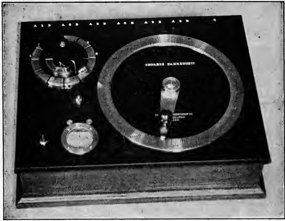
FIG. 67. — Wheat tone bridge indicator for platinum resistance pyrometer.
