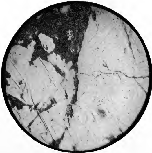
FIG. 100. — Copper matte. The light portion of the field is "D." The dark portion is "F," metallic copper.
