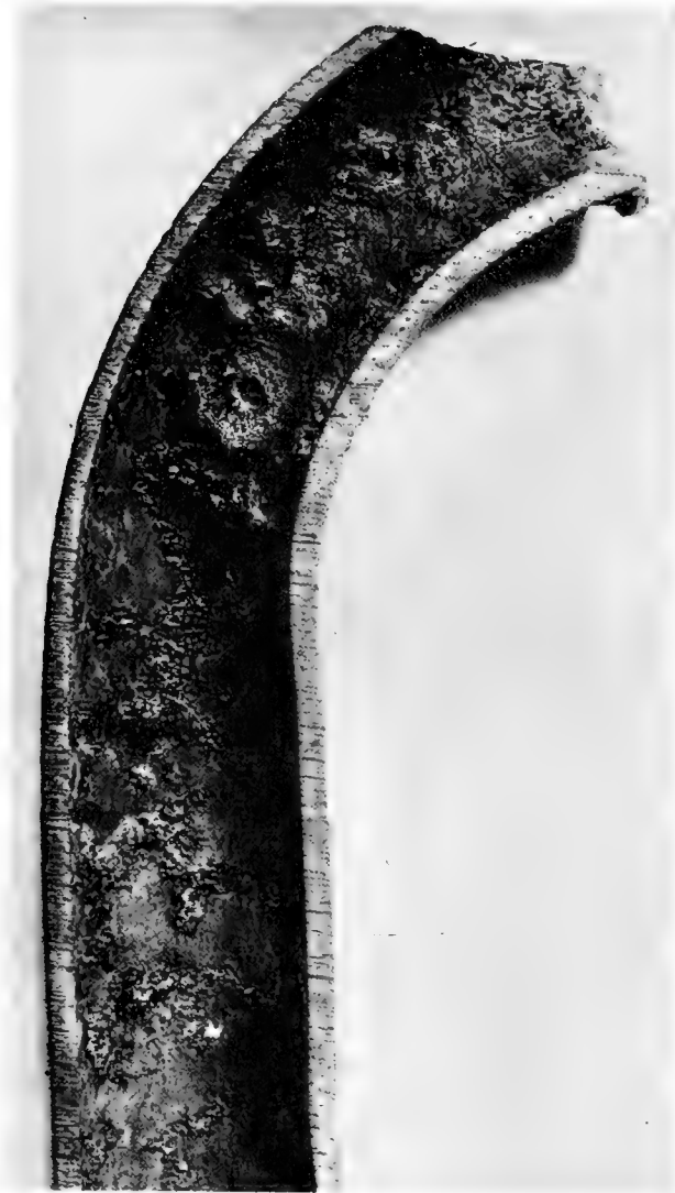
Figure 10-29.—Evidence of carryover in superheater tube.
