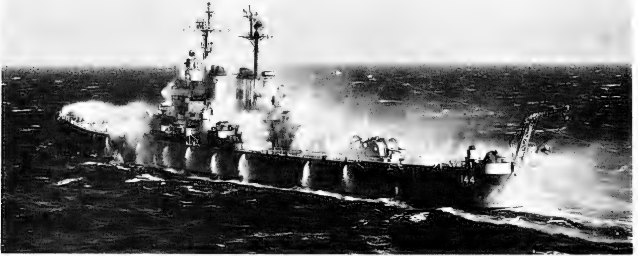
Figure 4-9.—Water washdown system in operation.
