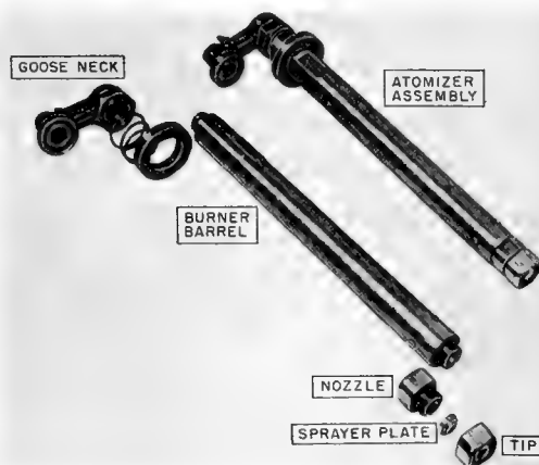
38.71 Figure 10-12.—Parts of a straight-through-flow atomizer assembly.
