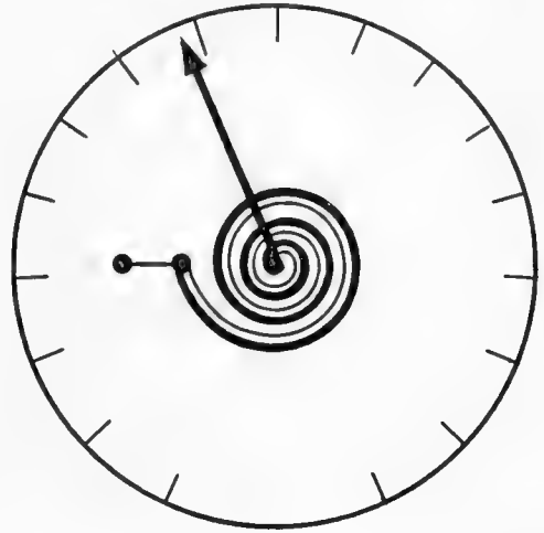
Figure 7-7.—Bimetallic thermometer (flat spiral element).
