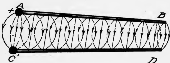
FIG. 23.—Electric field between two conducting rods.
