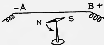
FIG. 16.—Magnetic effect of current-carrying wire.
