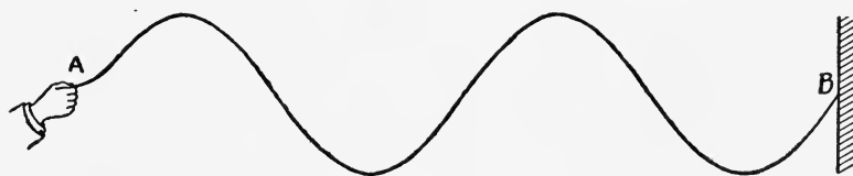
FIG. 38.—Wave motion in a rope.
