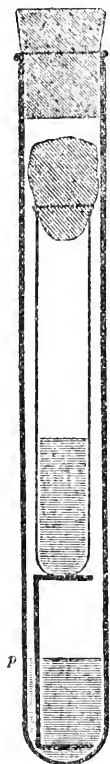
FIG. 9. Buchner tube for the anaerobic cultivation of bacteria: p , the alkaline pyrogallol solution; inner tube contains culture of organism (after Omeliansky).
