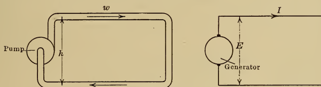
FIG. 21.—Hydraulic and electric circuits.
