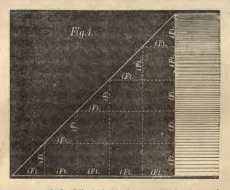
The pressure of the Mississippi then, on its banks—rejecting that from the blows of waves, or of currents—varies at the several depths as the widths vary in the above figure; and hence will that pressure be resisted effectively by any earthy matter, impervious to water, embanked in the above form.—Any earthy matter, provided it be impervious to water, piled up in the above form, will discharge the quiescent pressure of the water, because all earthy matter is heavier than water;
