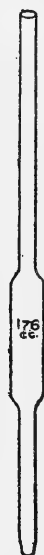
FIG. 34.—Pipette used in Babcock test for measuring milk. (From Chemical Testing of Milk and Cream, by R. H. Shaw, U. S. Dept. of Agriculture.)
