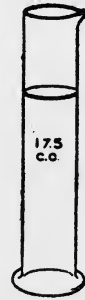
FIG. 35.—Cylinder used in Babcock test for measuring acid. (From Chemical Testing of Milk and Cream, by R. H. Shaw, U.S. Dept. of Agriculture.)
