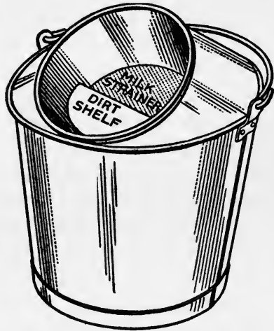
FIG. 14.—Covered-top pail with opening nearly horizontal (with strainer attached).
