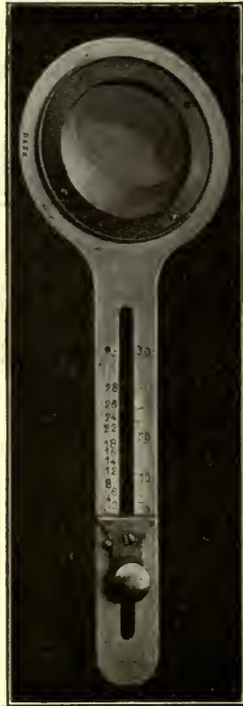
FIG. 65.—Front view of the revolving prisms as arranged by Crété.
