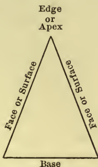
FIG. 4.—Principal section of a prism.
