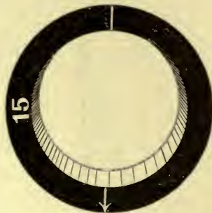
FIG. 9.—Prism with wide frame showing markings of base and apex and number on frame or cell.
