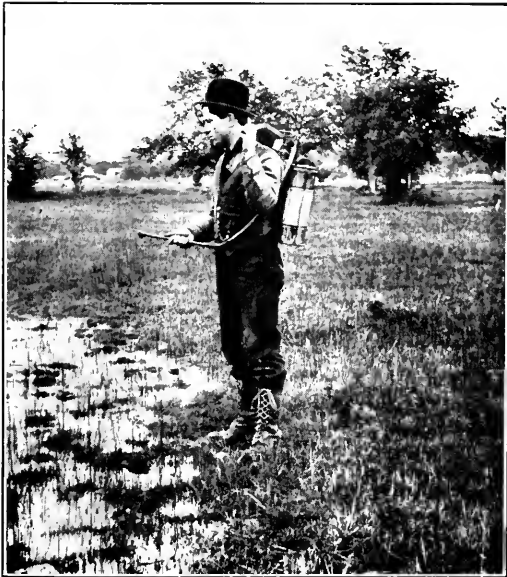
FIG. 2.—KNAPSACK SPRAY-PUMP IN USE, SPRAYING OIL ON A TYPICAL ANOPHELINE BREEDING PLACE.
