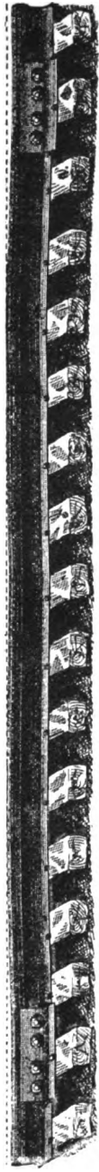
Cur No. 2. — Represents the Second Form of Permanent Set in Rails, low at the joints and centre and high at the quarters.
