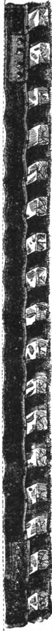
Cur No. 3. — Represents the Third Form of Permanent Set in Rails, a series of more or less irregular waves or bends.
