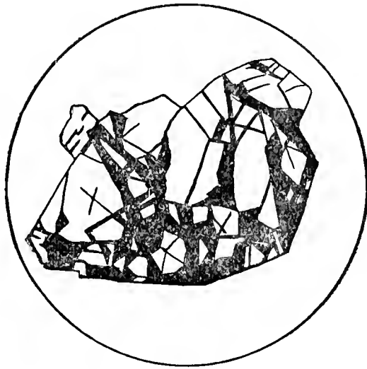
SECTION OF OLIVINE CRYSTAL SHOWING CHROMITE.
