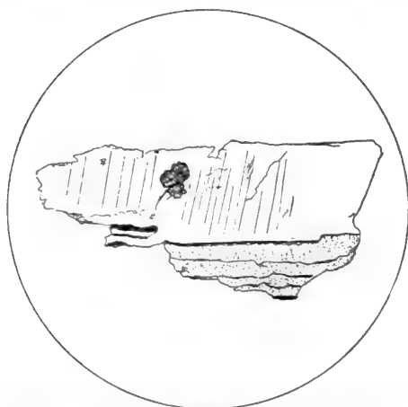
Fig. 21. Twinned crystal of labradorite, showing cleavage. \times 60 .
