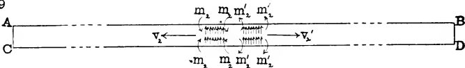
FIGS. 17-19.—Collision of Reflected Electric Flux Waves in Circuit of Perfect Conduction and Insulation Short-Circuited at Termini.
