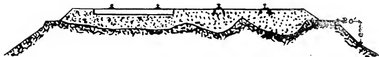
FIG. F—SECTION OF DOUBLE-TRACK ROADBED ON CLAY EMBANKMENT BUILT IN 1873, SHOWING DISTORTION BOTH UNDER CROSS-TIES AND LONGITUDINAL SLEEPERS.
