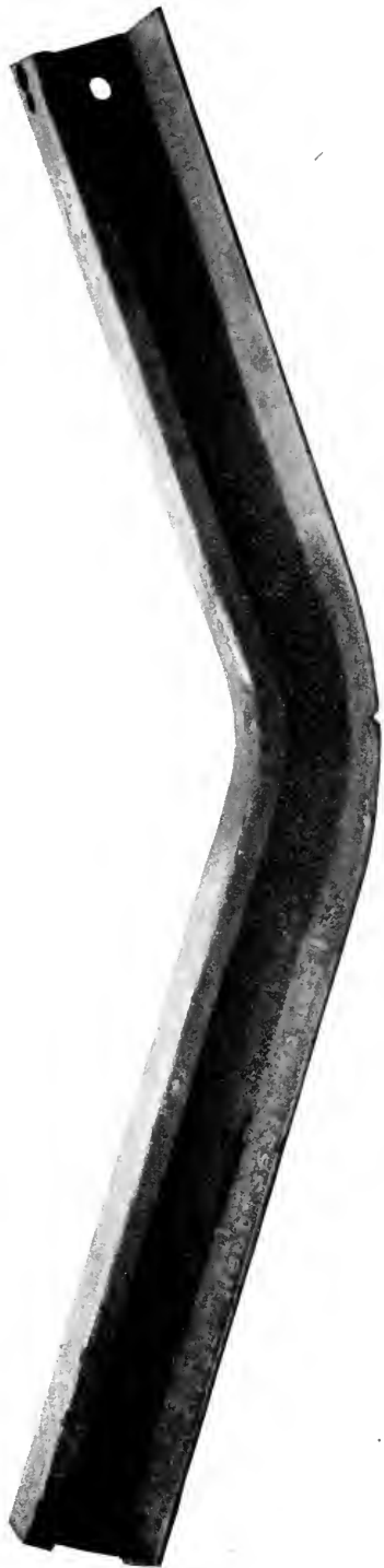
TEST No. 6-A. 85-Lb. A. S. C. E. SECTION "MANARD" RAIL, ROLLED AT STEELTON, P. S. Co. HEAT No. 3631.
