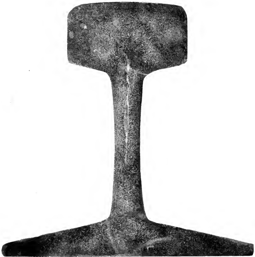
CHARGE No. 75828. TOP OF INGOT. TWO PER CENT. OF 10 PER CENT. FERRO-TITANIUM ADDED.
