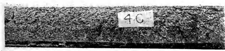
FIG. 32—VERTICAL LONGITUDINAL FRACTURE OF FLANGE, SHOWING LONGITUDINAL SEAM IN BOTTOM OF BASE.
