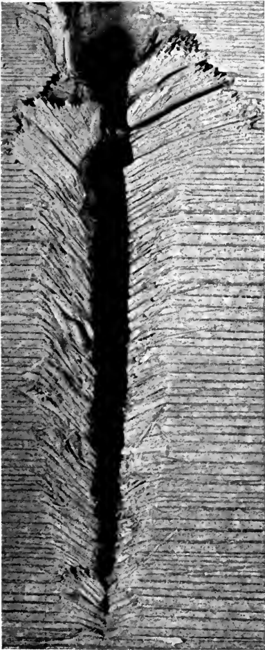
Chisel Point. Showing effects of cut spike inserted in redwood. No hole bored. Note badly broken fiber caused by chisel-point spike.
