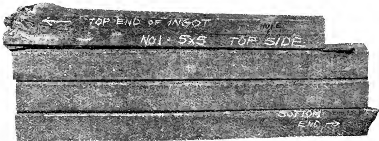
FIG. 7—TOP SIDE OF TOP QUARTER OF INGOT ROLLED INTO 5 X 5 INCH BLOOM. PICKLED.
