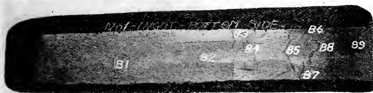
FIG. 10—BOTTOM SIDE OF INGOT SKINNED OFF IN PLANER.
