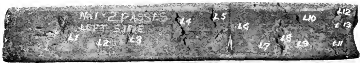
FIG. 25—LEFT SIDE OF INGOT AFTER TWO PASSES, MAKING LEFT SIDE OF BLOOM.
