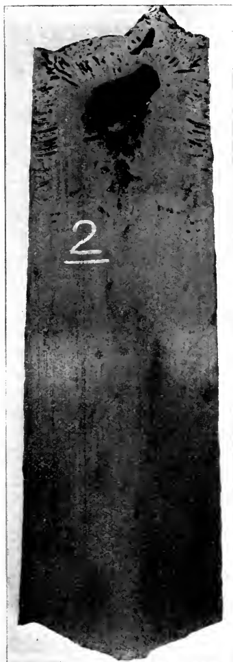
FIG. 2—INGOT No. 2, PLAIN BESSEMER STEEL.
