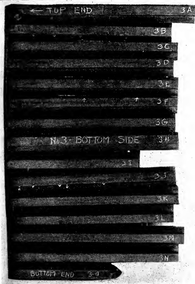
FIG. 14—BOTTOM SIDE OF THIRD QUARTER OF INGOT ROLLED INTO RAIL. MAKING TOP OF HEAD. PICKLED.
