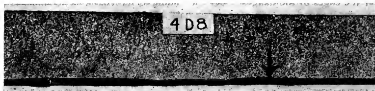
FIG. 10—VERTICAL LONGITUDINAL FRACTURE OF FLANGE, SHOWING LONGITUDINAL SEAM IN BOTTOM OF BASE.
