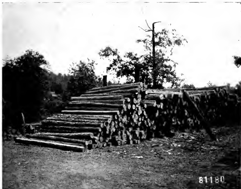
Plate II. Fig. 1.—Unpeeled Ties in Solid Piles. (In a warm, moist climate timbers piled in this manner are liable to insect attack and decay before they become seasoned.)
