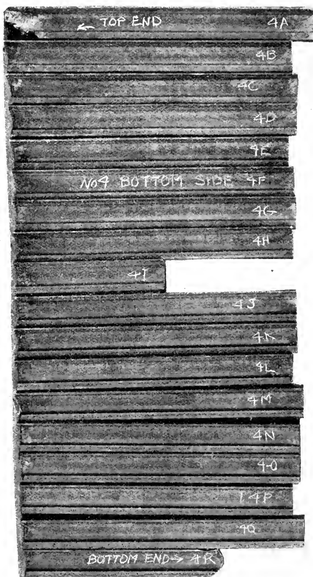
FIG. 15—BOTTOM SIDE OF BOTTOM QUARTER OF INGOT ROLLED INTO RAIL. MAKING RIGHT SIDE OF RAIL. PICKLED.
