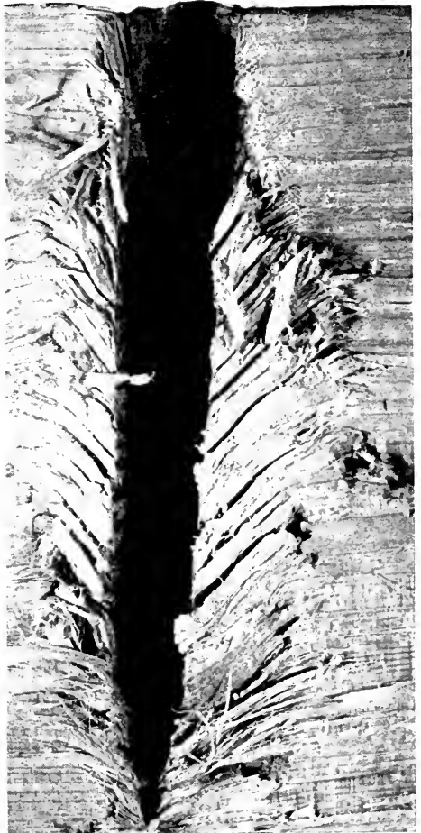
Chisel Point Spike. Showing effects of cut spike inserted in cedar; no hole bored. Note badly broken fiber caused by chisel point.
