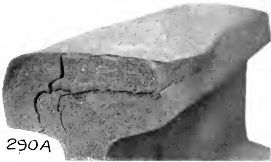
FIG. 290A. VIEW OF END OF "CRUSHED" HEAD RAIL 290.
