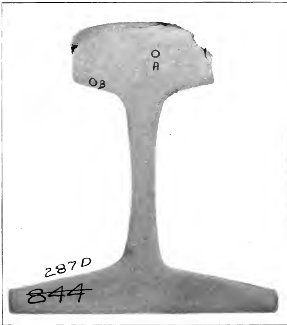
FIG. 287D. LIGHT ETCHING OF RAIL 287.
