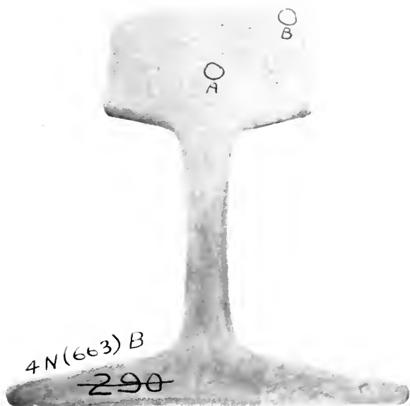
FIG. 4N(663)B. LIGHT ETCHING OF RAIL 663.
