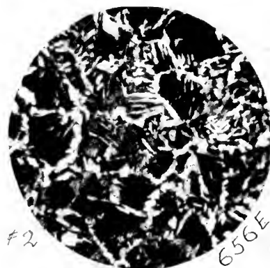
FIG. 656E. MICROPHOTOGRAPHS OF RAIL 656, MAGNIFIED 65 DIAMETERS, PRESUMABLY BELOW SURFACE. GENERAL STRUCTURE OF STEEL IN RAIL. (Both etched with nitric amyl alcohol.)
