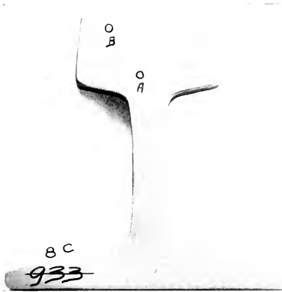
FIG. 8C. LIGHT ETCHING OF RAIL 8.
