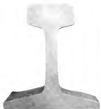
HEAT No. 5407, Ingot No. 15, SAMPLE No. 3, PHOTOGRAPH No. 1049. Etching of a section from bottom of A-rail. The fracture showed no sign of interior defect. Approximate distance from top of ingot, 10.6 per cent. Analysis Junction of Corner of head head and web Carbon by combustion 0.5 0.70 Per cent. of segregation 77
