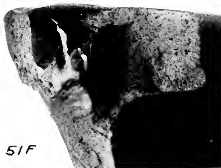
FIG. 51F. ANOTHER VIEW OF SPLIT IN HEAD OF RAIL 51.
