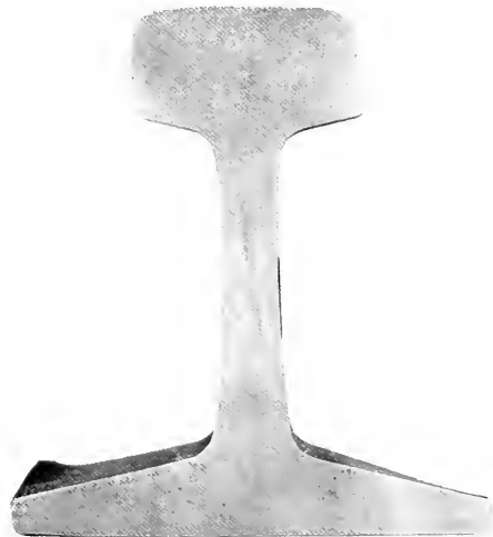
HEAT No. 7451, INGOT No. 11, SAMPLE No. 2, PHOTOGRAPH No. 1054. Etching of a section 4 ft. from top of "A" rail. Showed segregated on fracture. Approximate distance from top of ingot, 14.5 per cent.
