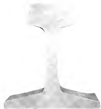
HEAT No. 5407, Ingot No. 15, SAMPLE No. 2, PHOTOGRAPH No. 1048. Etching of a section from middle of A-rail. The fracture showed no sign of interior defect. Approximate distance from top of ingot, 21.4 per cent. Analysis Junction of Corner of head head and web Carbon by combustion 0.25 0.8 Per cent. of segregation 88
