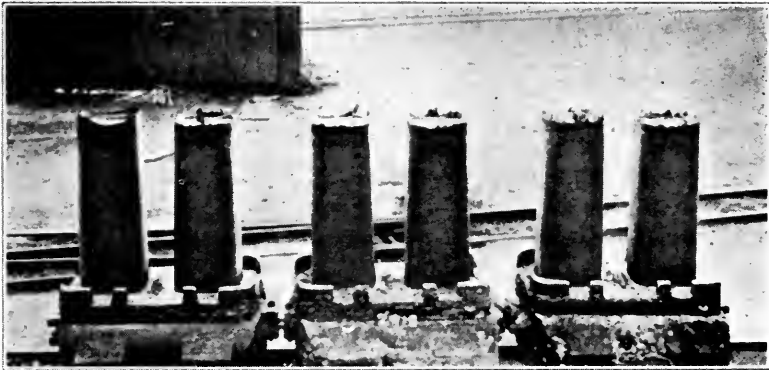
FIG. 90. REPRODUCTION OF A PHOTOGRAPH TAKEN MARCH, 1908, OF A HEAT OF RED HOT INGOTS, 19 IN. BY 19 IN., ON BASE, WITH CORNER RADIUS OF 3\frac{3}{4} IN. FOR THREE LENGTHS OF 100-LB. 33-FT. RAILS, WITH SMOOTH, FLAT TOPS. LACKAWANNA STEEL COMPANY, BUFFALO, N. Y.
