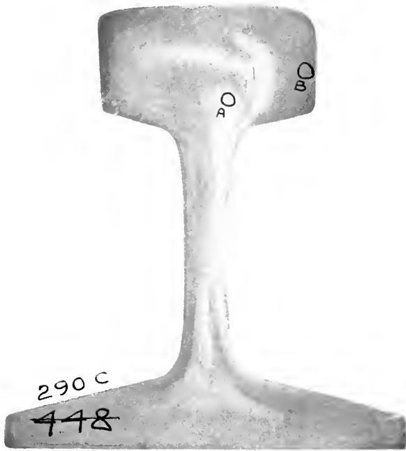
FIG. 290C. LIGHT ETCHING OF RAIL 290.
