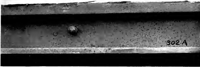
FIG. 302A. SHOWING "FLOW OF METAL" OF RAIL 302.
