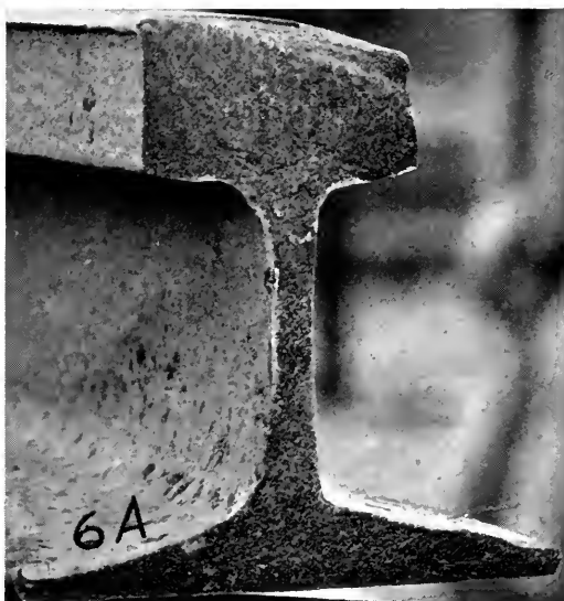
FIG. 6A. FRACTURE OF "BROKEN" RAIL 6.
