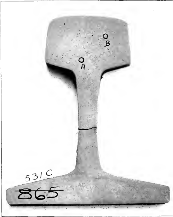
FIG. 531C. LIGHT ETCHING OF RAIL 531.
