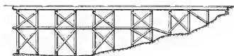
Longitudinal Bracing on Frame Trestles Frame trestles to have long bracing for all heights.
