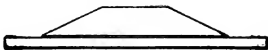
(a) Pat with Top Surface Flattened for Determining Time of Setting by Gillmore Method
