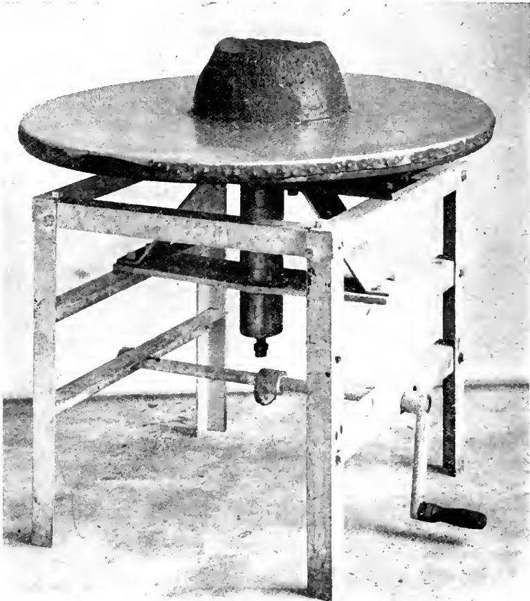
FIG. 7—BUREAU OF STANDARDS FLOW-TABLE FOR CONSISTENCY OF CONCRETE.
