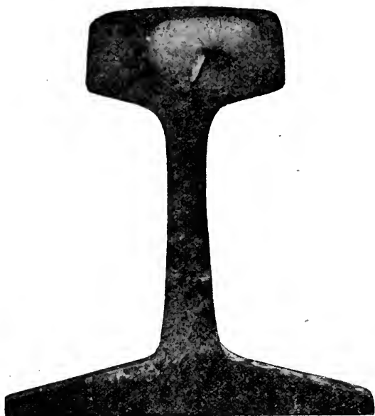
FIG. 1—INTERIOR TRANSVERSE FISSURES, INTERGRANULAR TYPE, NUCLEUS OVER OUTSIDE OF WEB. ONE-HALF SIZE, 6-INCH 100-LB. RAIL.
